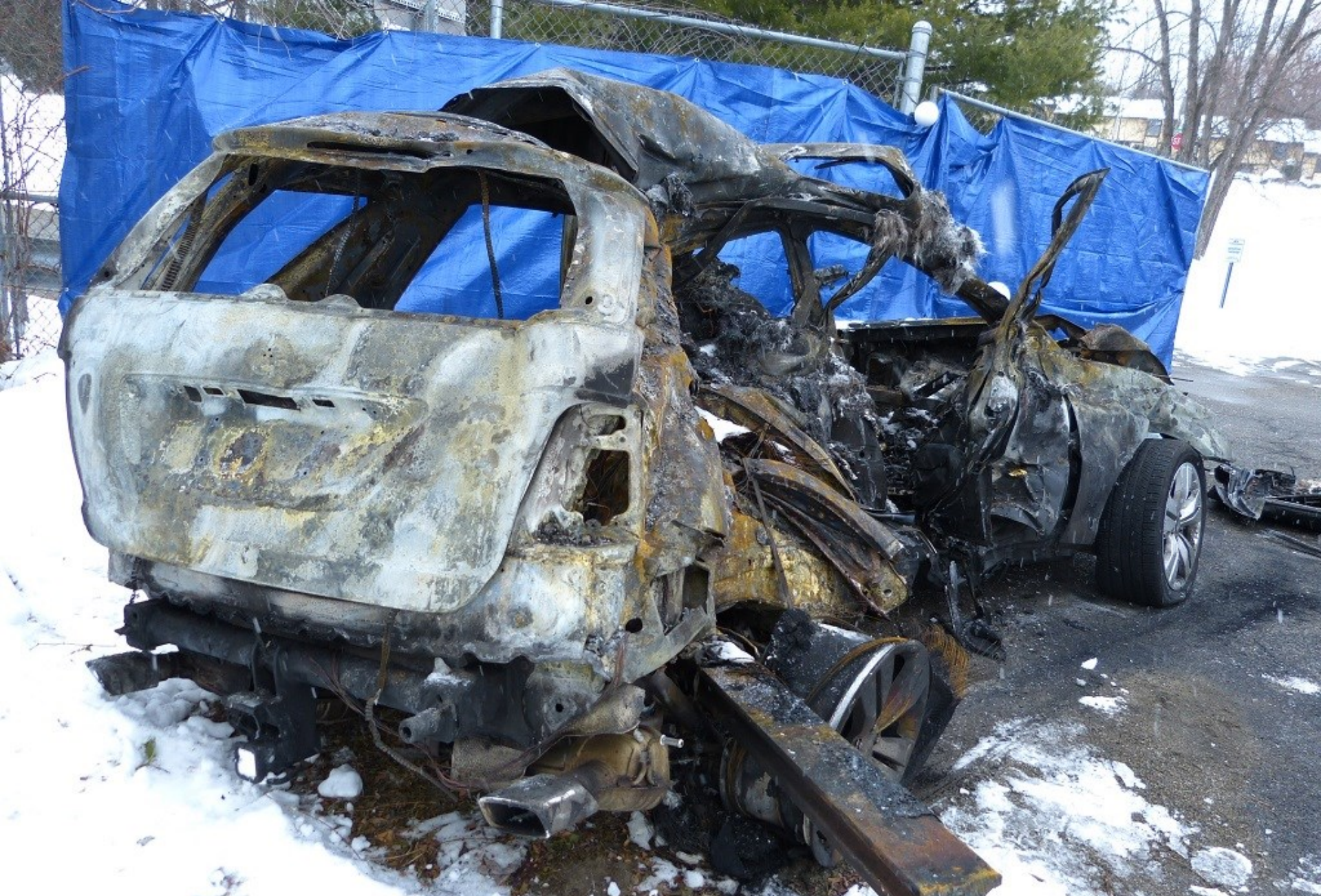
The rear and a portion of the right side of the SUV is visible. The railroad rail protruding from the right rear corner of the car is visible and the severe crushing of the right side of the car is visible.
