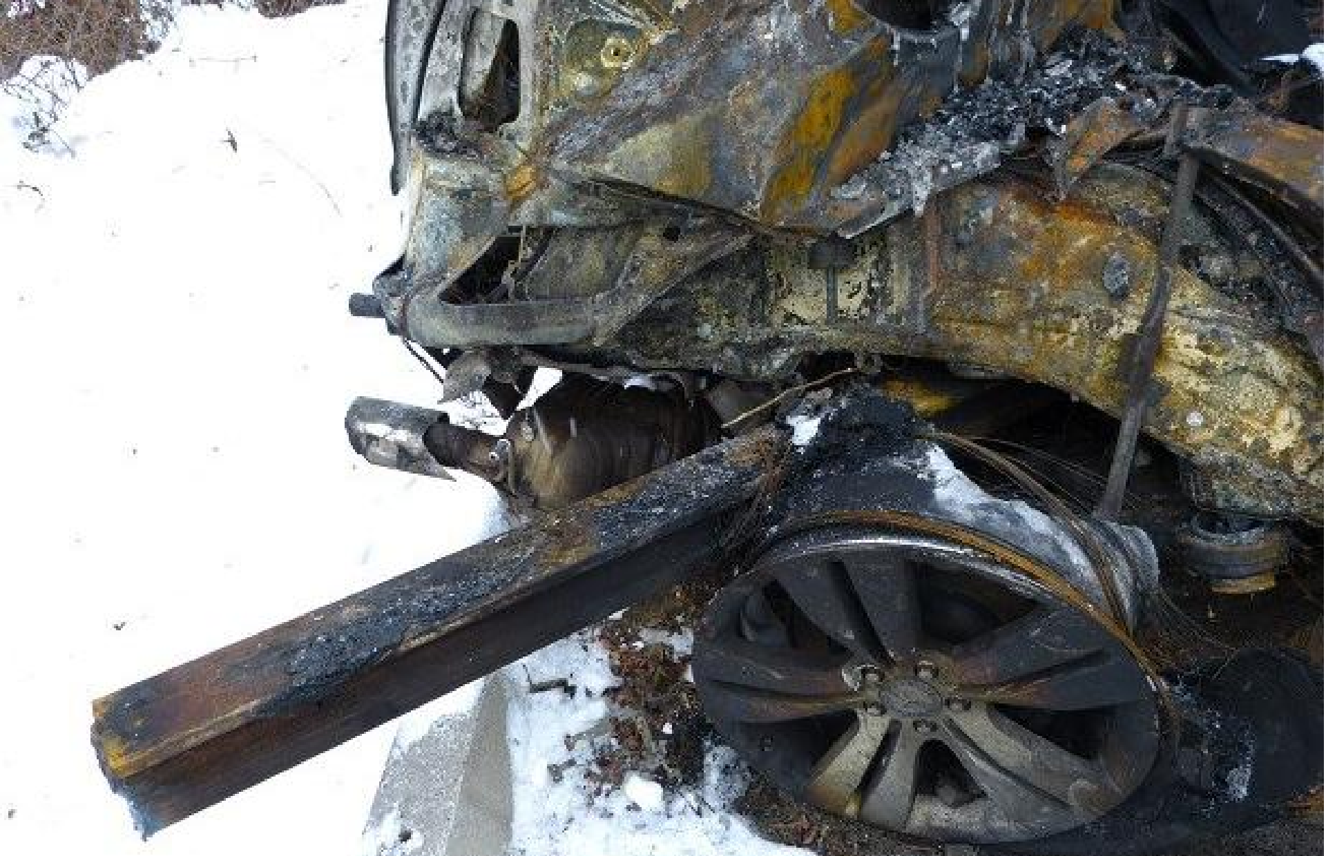
Details of the lower right rear portion of the SUV are visible. The right rear wheel with burned away tires and damaged right rear quarter panel are visible. A section of third rail is protruding from the upper left corner of the wheel well, and is in contact with the wheel.
