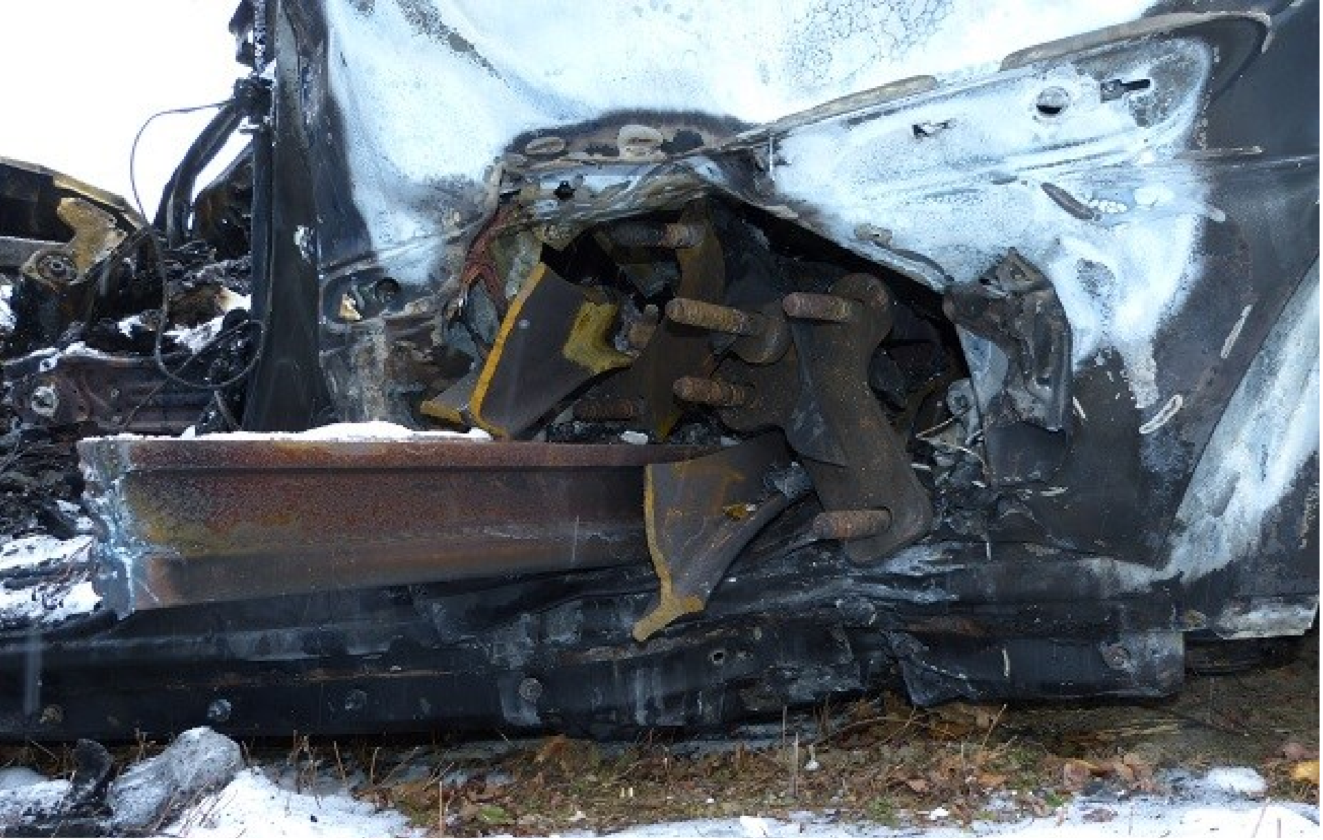
A detail view of the lower left side rear door section of the SUV is visible. A section of railroad rail and railroad brackets are visible protruding from the car just above the floorpan and in front of the left rear wheel.
