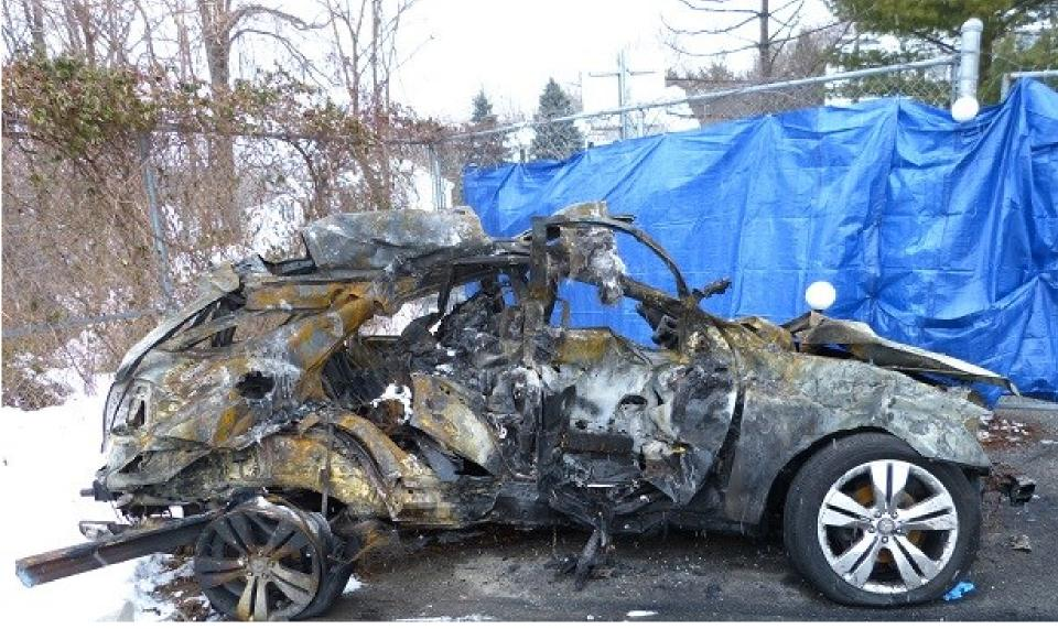
The right side of the SUV is shown. The vehicle is badly fire damaged and the middle portion of the car between the wheels in crushed inward. The fire damage is slightly less severe at the front, with the right front tire and wheel intact, but the tire is deflated. The right rear tire is burned away and the wheel is discolored. At the top left corner of the wheel there is a section of railroad rail visible, protruding from the side of the car.
