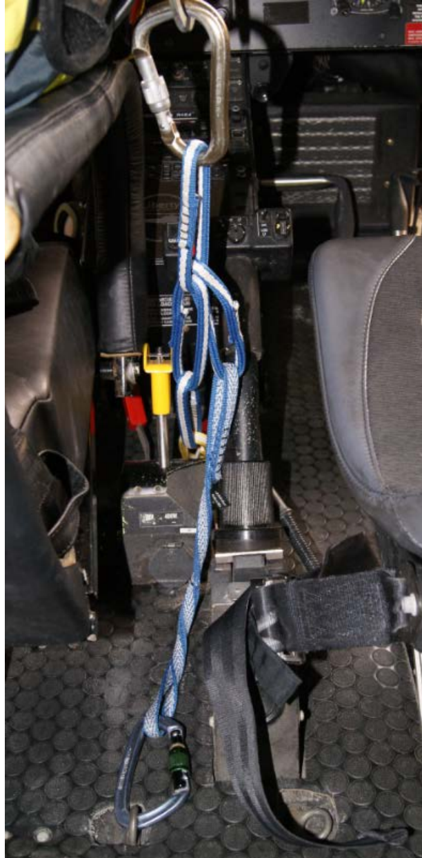
Photograph 20- Front seat occupant's tether showing additional tail length (4 loops) resulting from positioning of the carabiner within the attach loop (aft looking forward).
