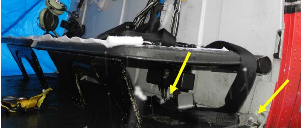
Photograph 9 - Lapbelts connected to the floor anchors/hard points adjacent to the rear bulkhead.
