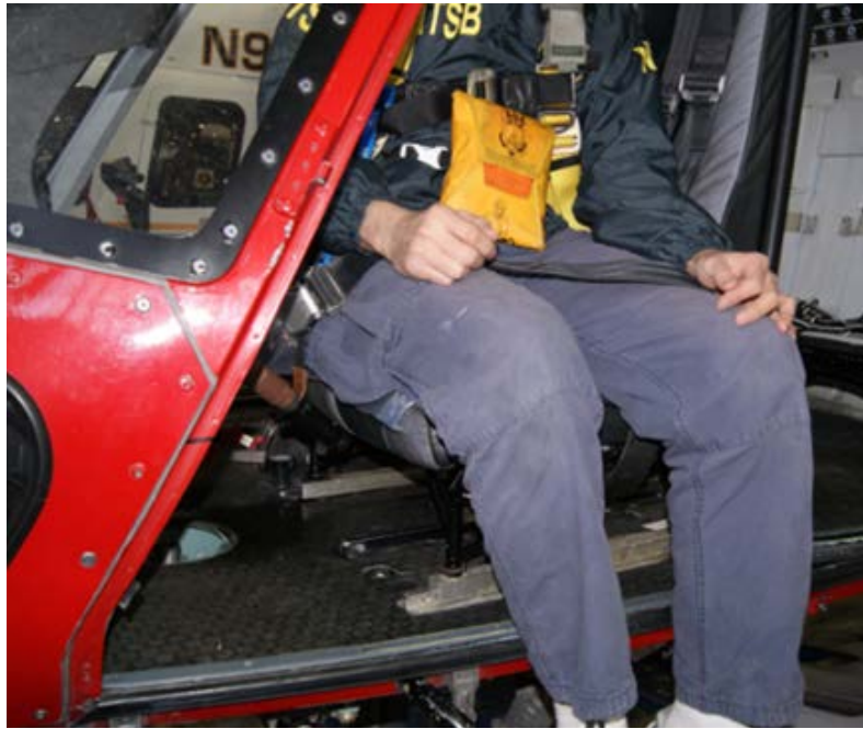
Photograph 23- Male subject seated upright in position to take a “shoe selfie” while wearing the FAA-approved restraints and harness/tether system.
