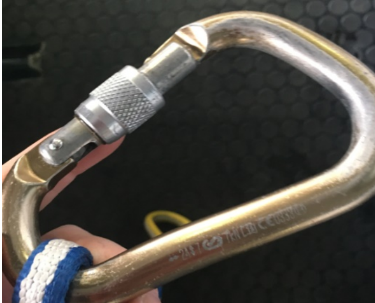
Photograph 27- Silver screw gold body carabiner (Label 24/7/7kN CE0333).
