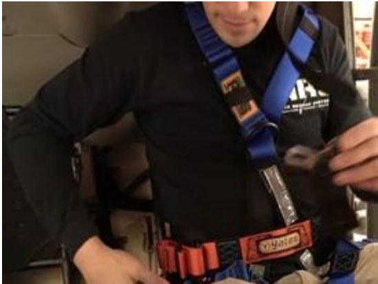
Photograph 46 – Screen captures from NYONair’s video submission to the FAA showing use of Air Rescue Systems (ARS) 339 Heli-Ops Harness with the ARS Personal Retention Lanyard with Quick Release Device and the FAA approved seatbelt.
