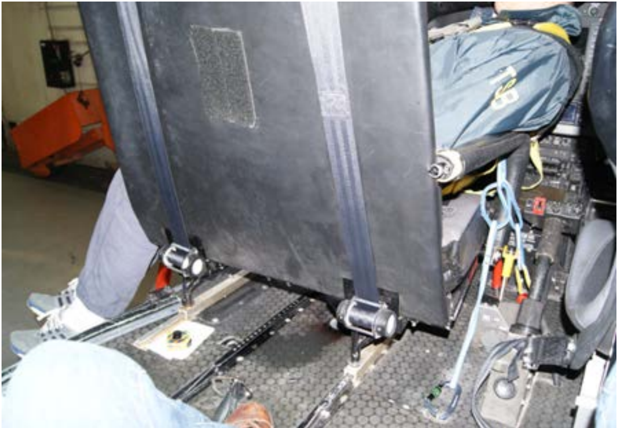
Photograph 24- Male subject in front seat reclined in position to take a “shoe selfie” with tether tail loops visible.
