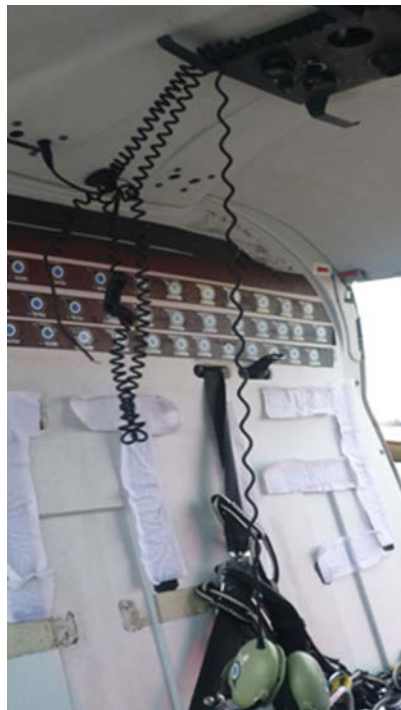
Photograph 42 –Headset coiled cord connected to overhead audio panel.
