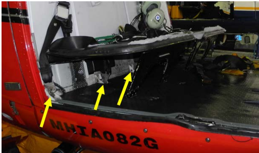
Photograph 8 - Lapbelts connected to the floor anchors/hard points adjacent to the rear bulkhead.
