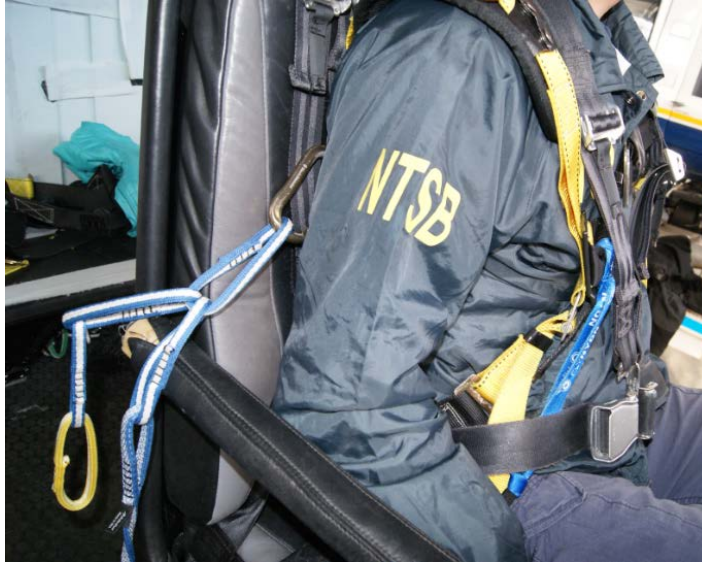
Photograph 21- Front seat occupant's tether routed over the armrest.
