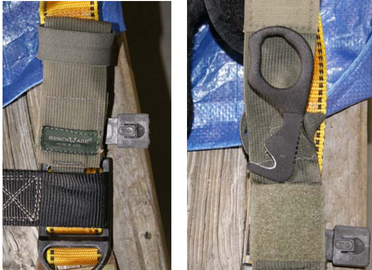
Photograph 36- Harness A cutter (Benchmade olive green pouch with a Benchmade Model 7 rescue cutter).
