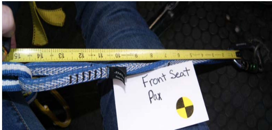
Photograph 19- First long blue loop of front seat occupant tether.
