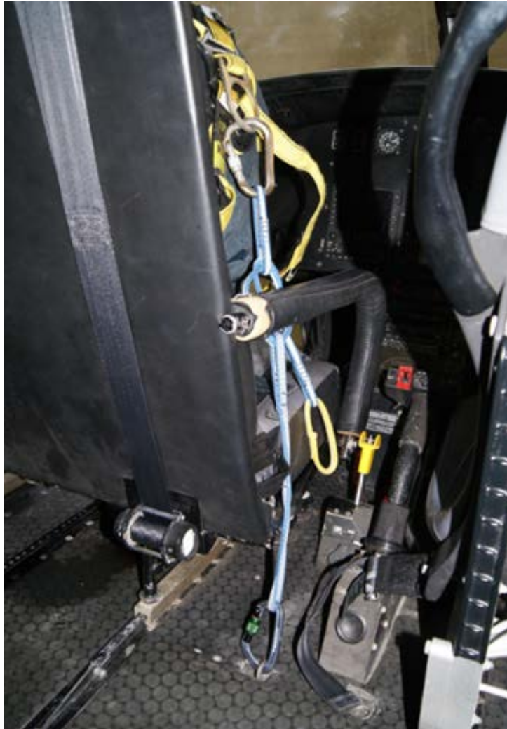
Photograph 22- Front seat occupant tether routed under the armrest.
