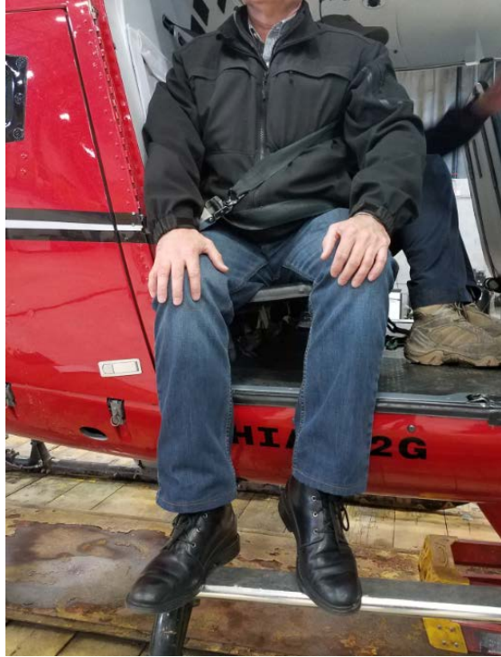
Photograph 6- Picture showing FAA approved shoulder harness restraint routed under the arm.
