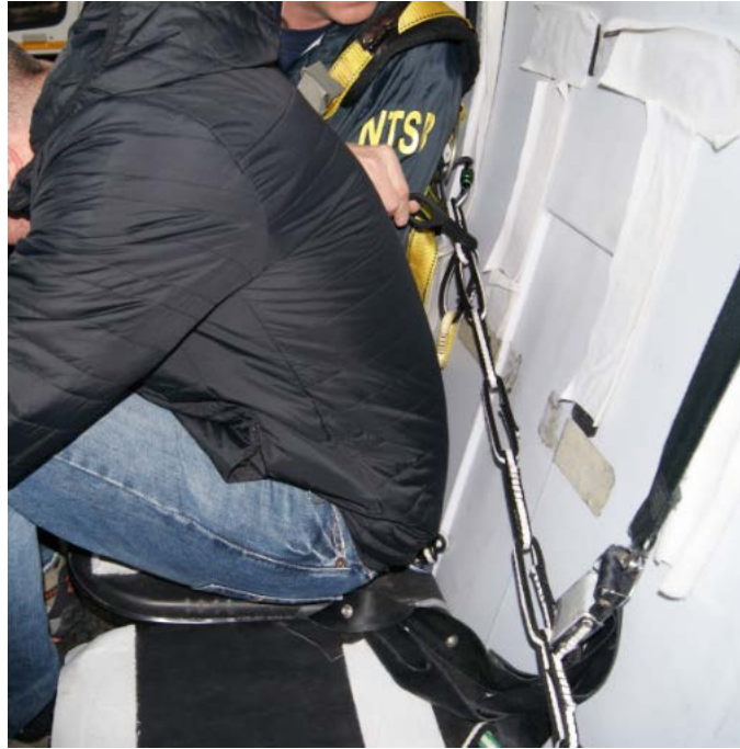
Photograph 39- NTSB investigator wearing the harness/tether system attempting to cut the tether with the cutter with another investigator seated beside him leaning forward to facilitate access to the tether.
