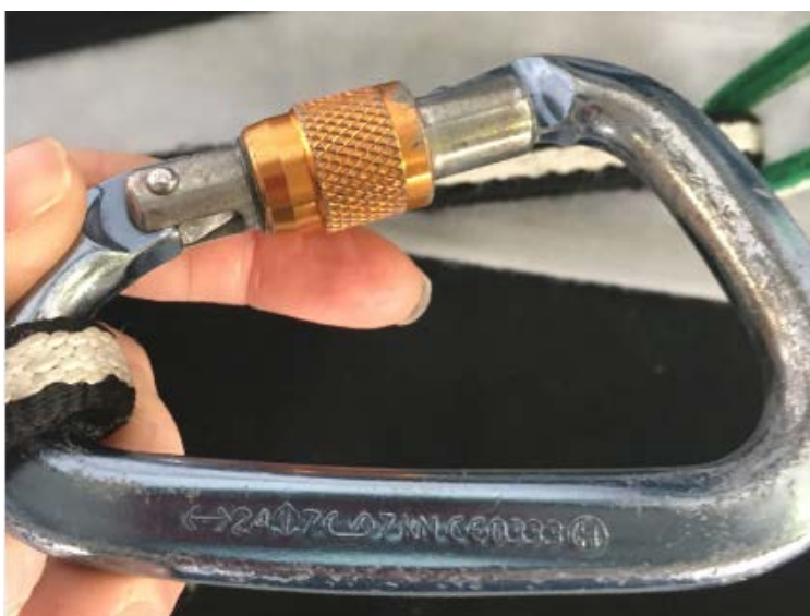
Photograph 26- Orange screw silver body carabiner (Label 24/7/7kN CE0333).
