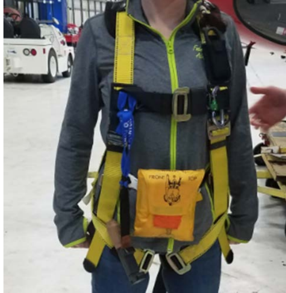
Photograph 40- PFD positioned around a passenger with the harness.
