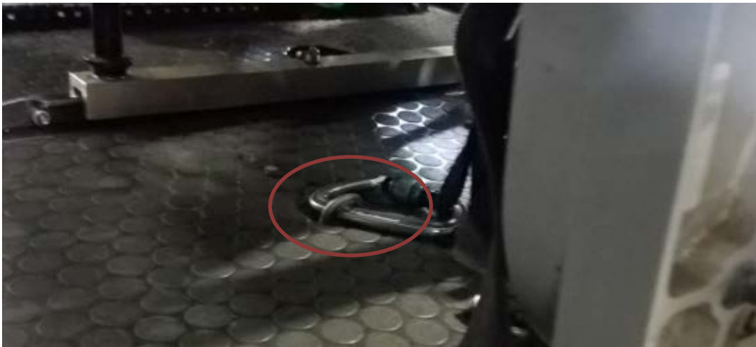
Photograph 12- Carabiner attaching tether to the front seat floor hard point in helicopter.
