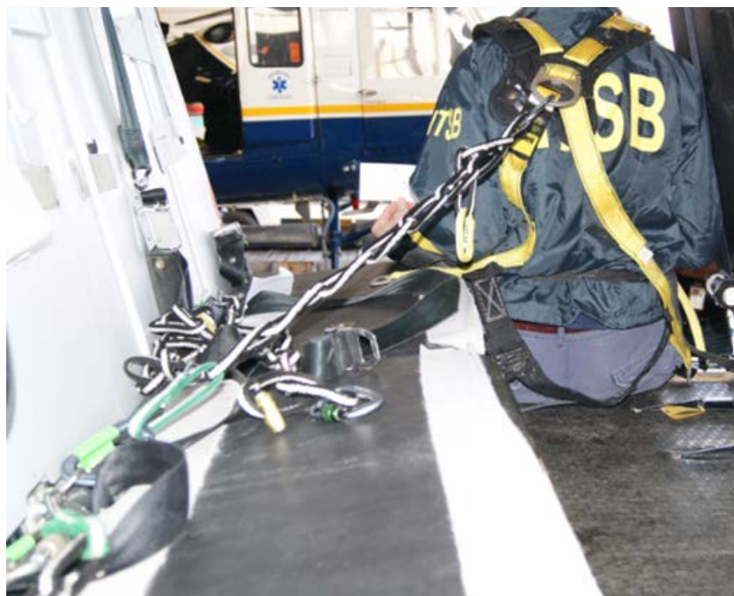
Photograph 15- Investigator seated on left doorsill wearing harness connected to tether (Tether number 2 attached to the hardpoint at seat position 3).
