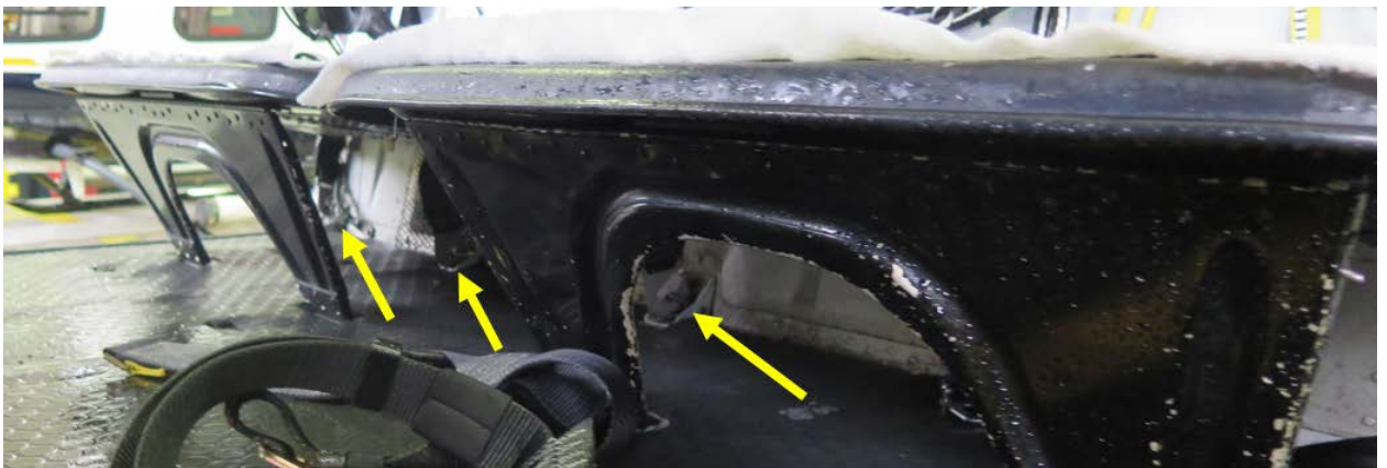
Photograph 10 - Floor anchors/hard points adjacent to the rear bulkhead
