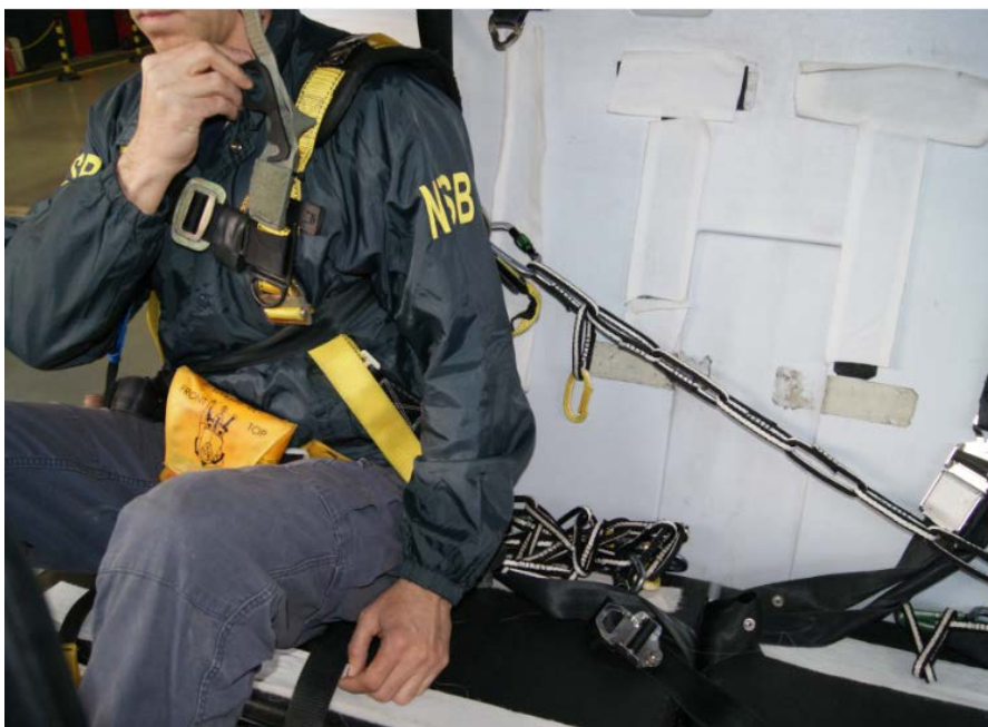
Photograph 38- Investigator wearing the harness/tether system removing the cutter from its stowage pouch.
