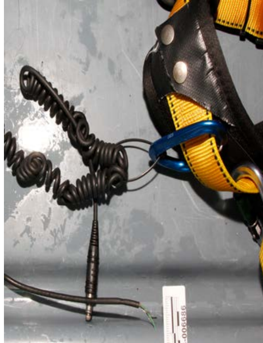
Photograph 41 –Headset cord connected to harness using zip ties and carabiner.
