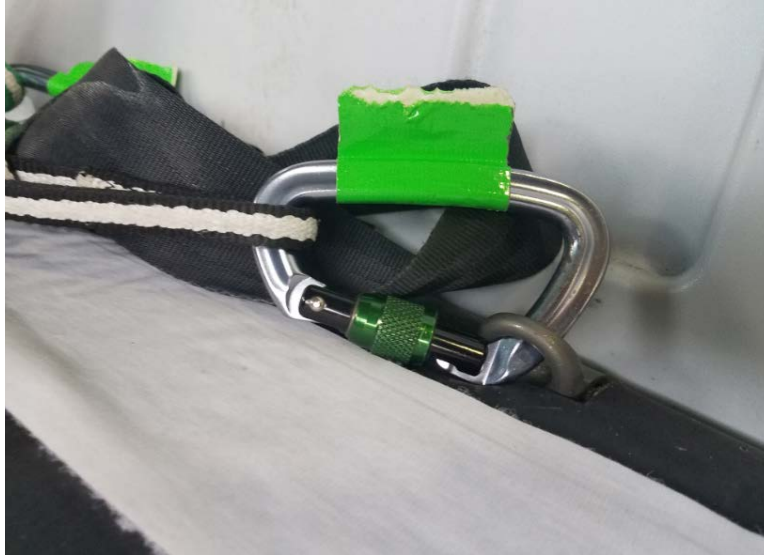
Photograph 11- Carabiner attaching tether to a rear bench seat tube hard point in helicopter.
