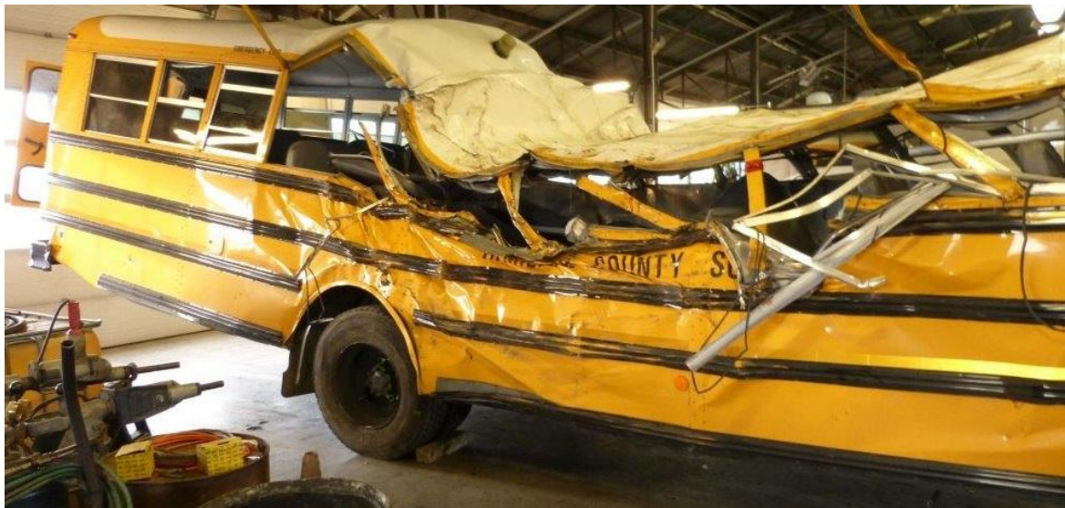
SF Photograph 4 shows a right rear view of the school bus. Severe damage to the upper portion of the middle of the bus is visible. The roof is crushed downward in the region above and forward of the rear axle. The crush is most severe just forward of the rear axle and decreases further forward. The passenger window frames above and forward of the rear axle are crushed. The portion of the bus aft of the rear wheels exhibits minor damage.
