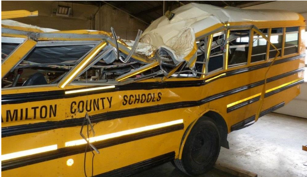
SF Photograph 3 shows a left rear view of the school bus. Severe damage to the upper portion of the middle of the bus is visible. The roof is crushed downward in the region forward of the rear axle. The passenger window frames forward of the rear axle are crushed. The portion of the bus aft of the rear wheels exhibits minor damage.
