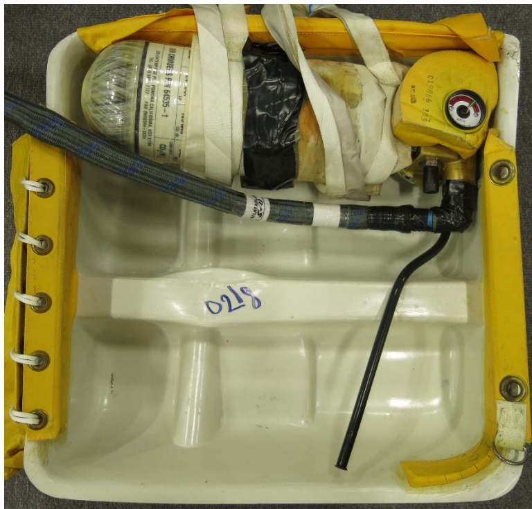
Photograph 3 – Reservoir and valve assembly (RVA) in slide packboard.
