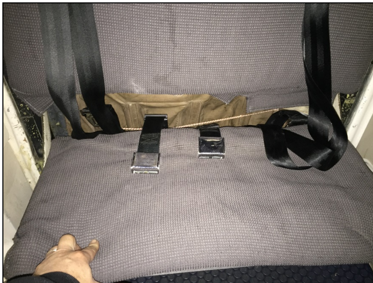
Photograph 2 – Tailcone jumpseat with both seat belts unbuckled.
