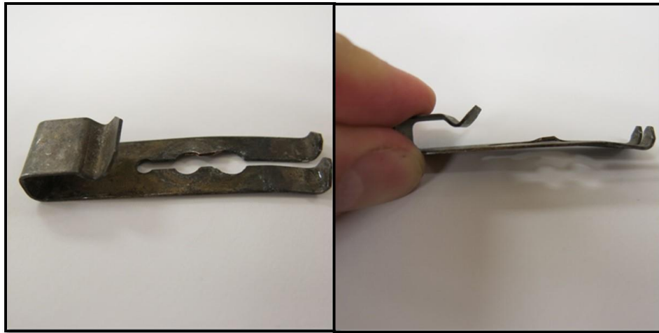
Photograph 13 – Top and side view of the retainer spring.
