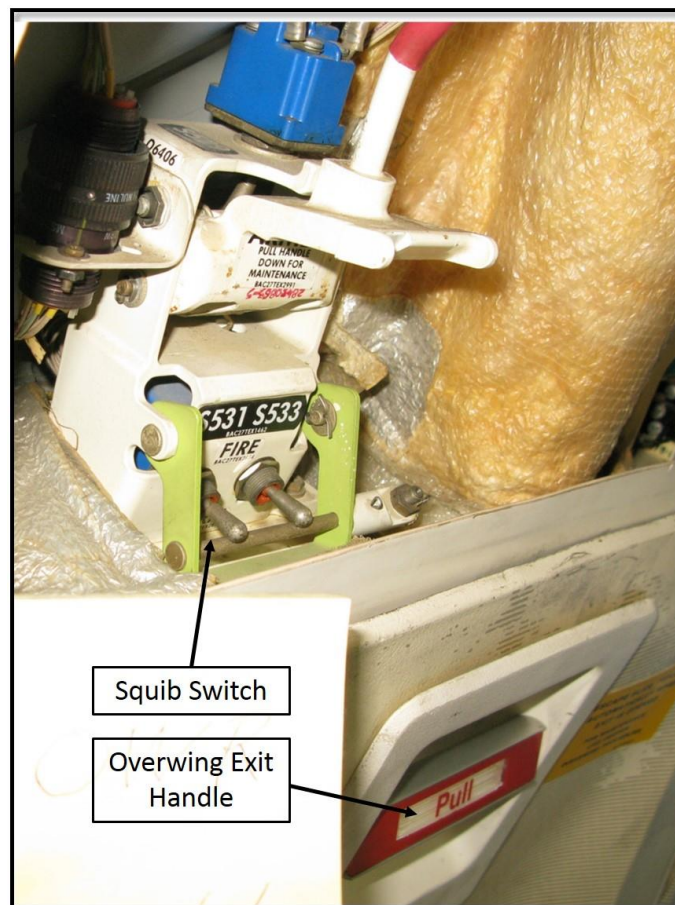
Photograph 1 – Right side squib switch and exit handle.
