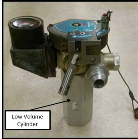
Photograph 11 – Regulator valve installed on low volume cylinder.
