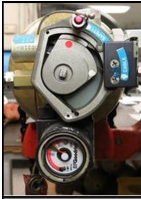
Photograph 9 – Regulator valve with cover plate removed.
