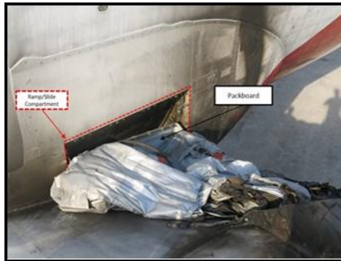
Photograph 3 – Left ramp/slide compartment with top portion of the ramp/slide and packboard.
