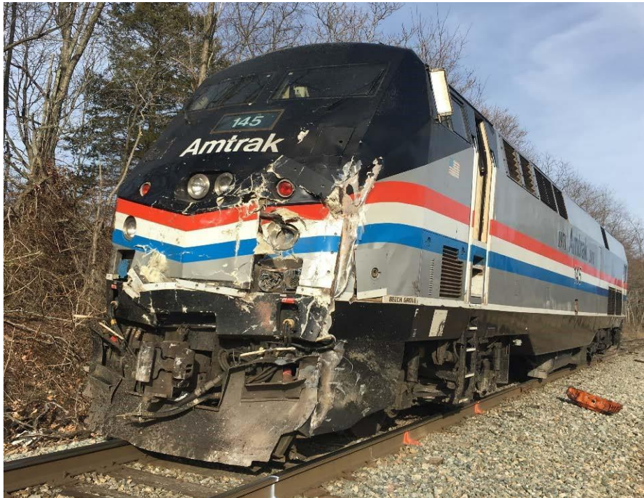
Photo #1: FBI photo showing exterior damage to lead locomotive.
