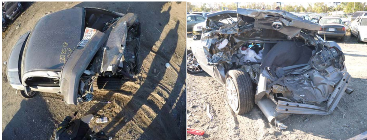
Figures 3a and 3b. Overhead view of deformation to back end of Mustang and left rear angle view of deformation.
