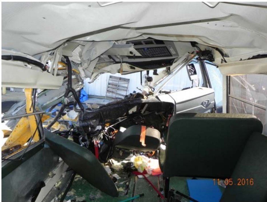
Figure 2. Interior view of intrusion to driver seating in the school bus.
