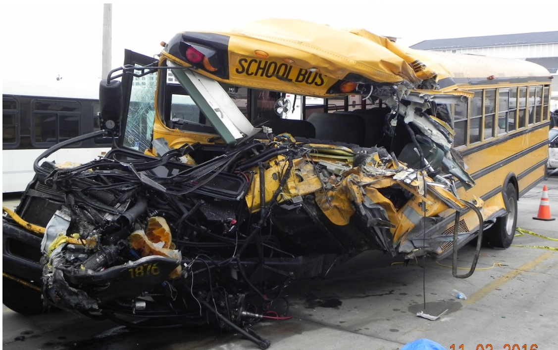
Figure 1. Exterior view of deformation to front end and left side of the crash involved school bus.
