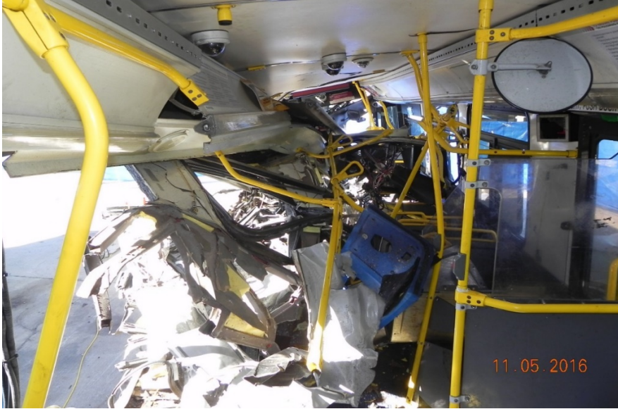
Figure 5. Interior view looking from rear to front showing extent of intrusion into occupant compartment in the crash involved transit bus.
