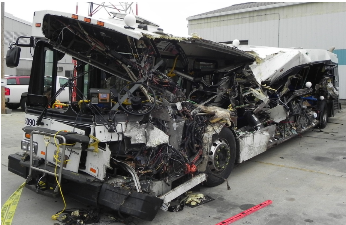
Figure 4. Exterior view of extent of deformation to front left bumper corner and down left side of New Flyer transit bus.
