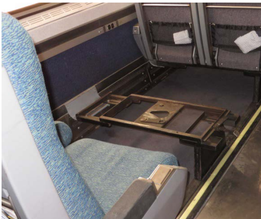
Figure 26. The row 12 seat frame.
