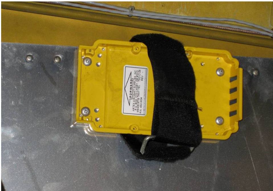
Photograph 2. ELT tray mounted on sidewall of accident airplane.
