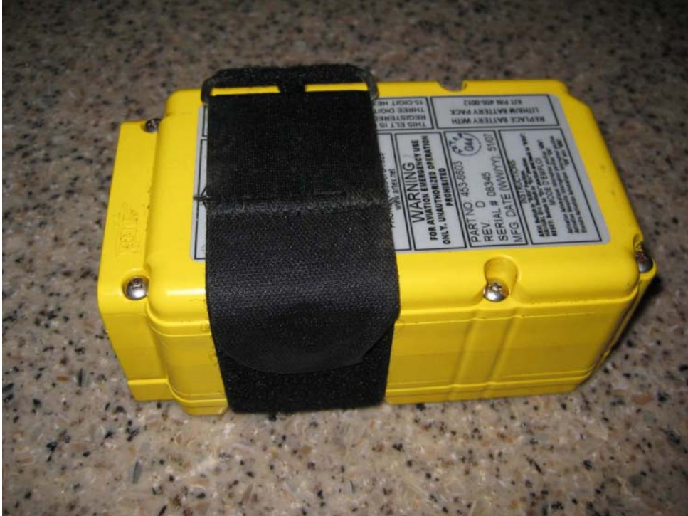
Photograph 1. Artex ME406 ELT in mounting tray, secured by Velcro strap.
