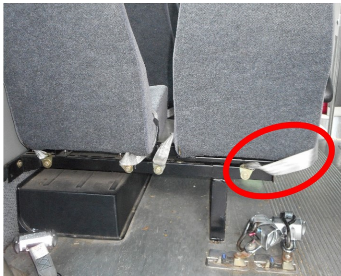
Figure 8. View of belt positioning to side (highlighted in red) in sister vehicle when side slide mechanism is utilized.
