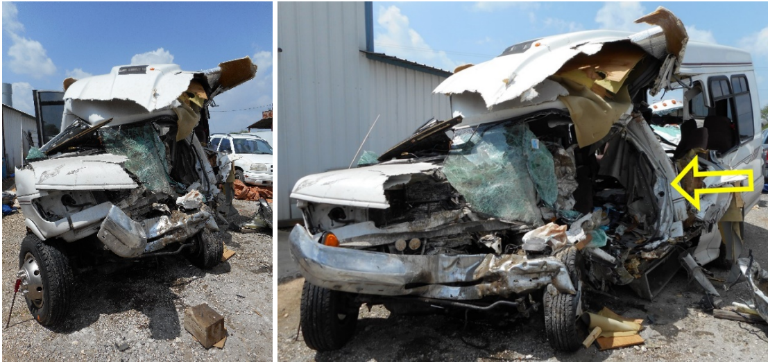
Figures 3 and 4. Photo on left is a frontal view and photo on right is a front left angle view of deformation to front end of Ford E350 bus. (Note; yellow arrow indicates area of accordion style crush to B-C pillars)
