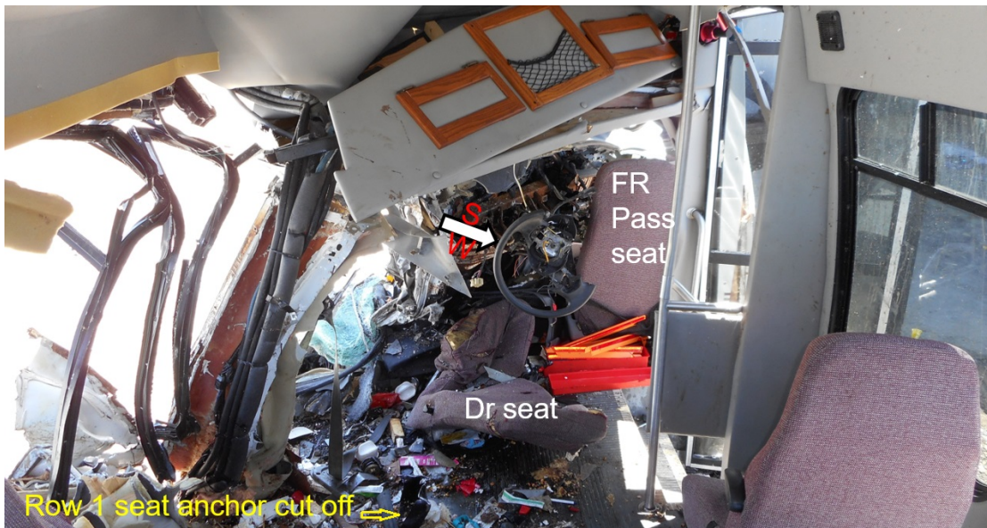
Figure 5. Interior view of Ford E350 from rear looking forward at interior intrusion and deformation. NOTE: Row 1 cut out during extrication process. Above abbreviations, SW is Steering Wheel, Dr = Driver, and FR = Front right passenger.
