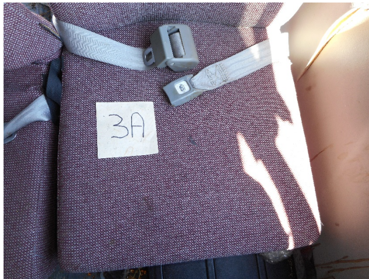
Figure 6. View of lap belt in seat 3A showing the “web winder” with latch and buckle.
