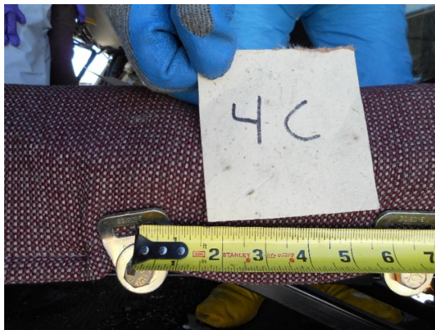
Figure 7. Close-up view of lateral lap belt attachment points on seat frame in row four.
