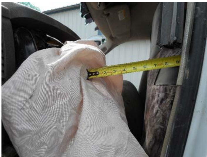
Figure 2. Close-up view showing drivers steering wheel approximately 7 inches from the center of the steering wheel to the drivers seatback.
