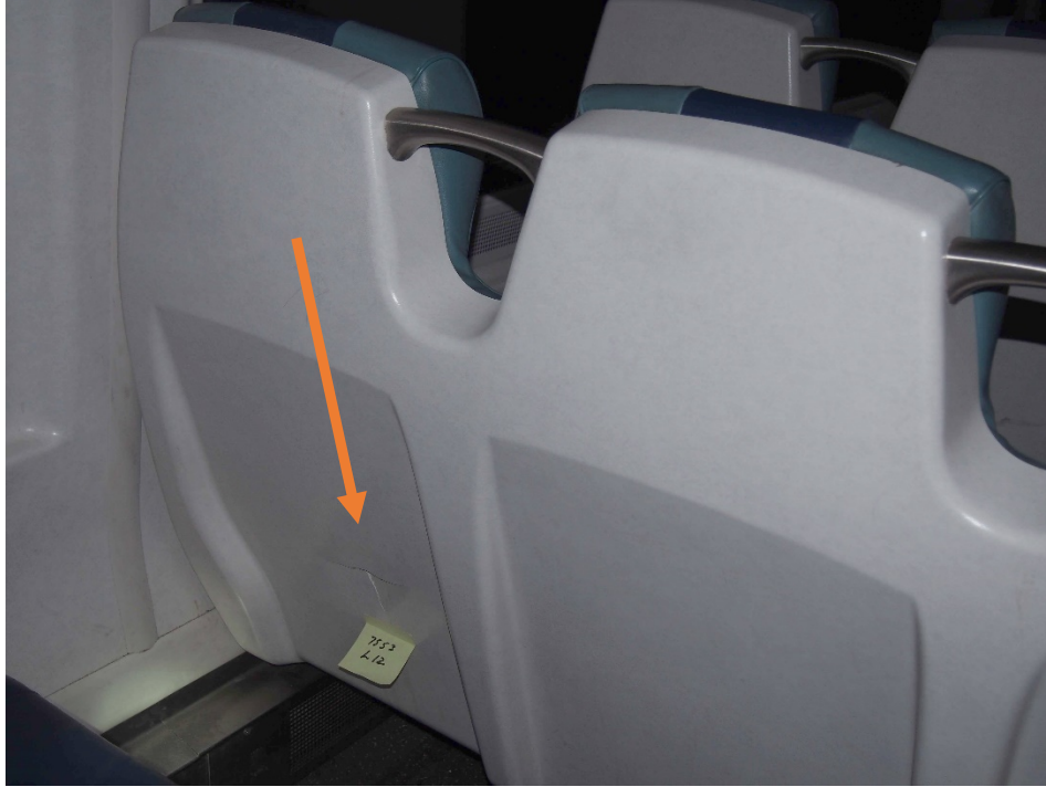
Figure 4- An example of a cracked seatback
