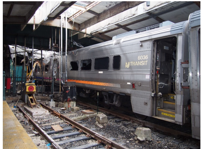
Figure 3- A view of the left side of the cab car and an exemplar bumping post on an adjacent track
