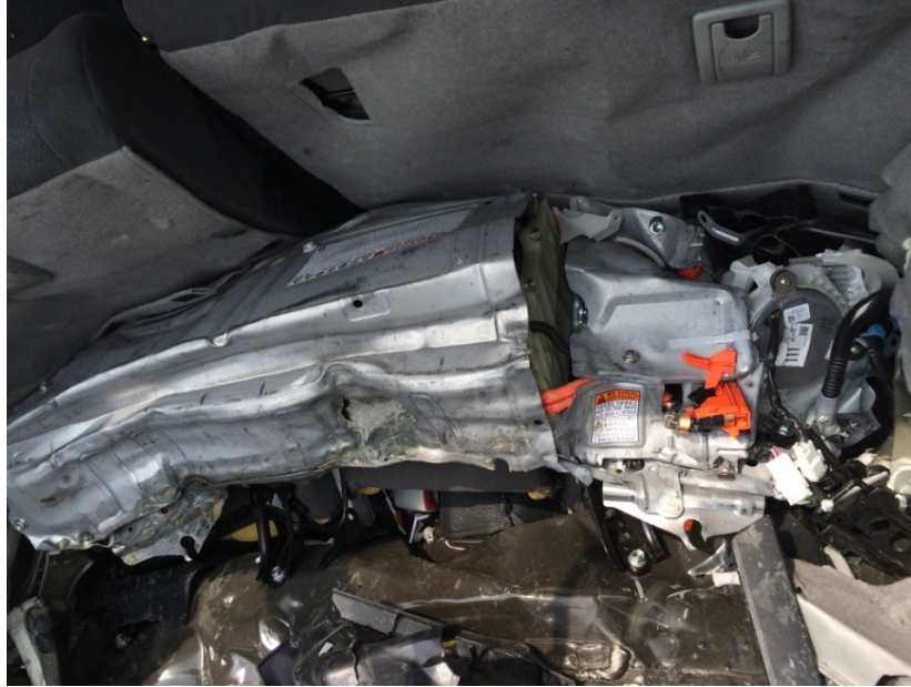
Figure 1. Cargo Area of the Prius with Damaged Battery Pack
