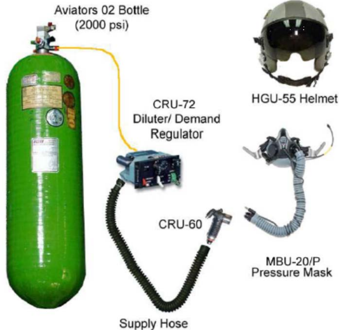
Figure 2. SS2 ECS components.
