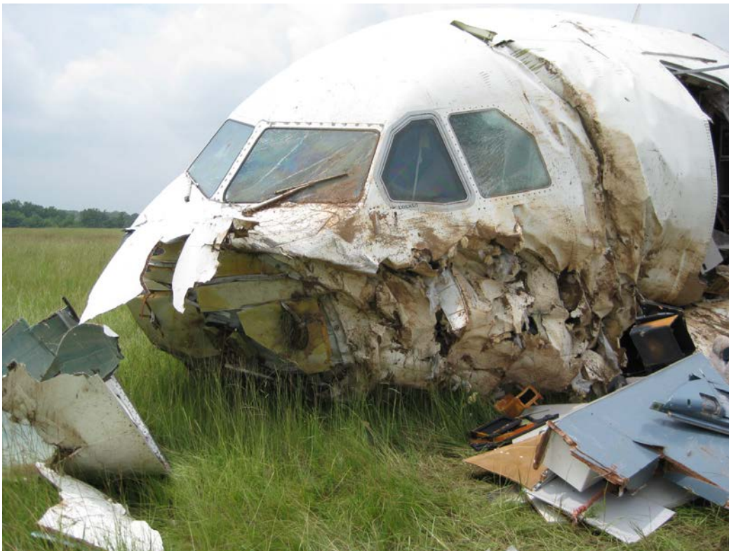
Photo 2. Damage under flight deck.
