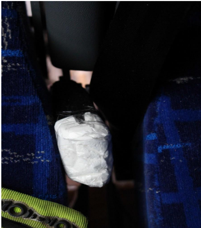
Photo #10: Taped defective seatbelt buckle on motorcoach
