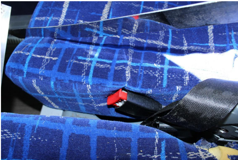
Photo #14: Defective seatbelt buckle for window seat
