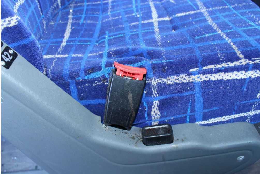
Photo #11: Defective aisle seatbelt buckle on motorcoach
