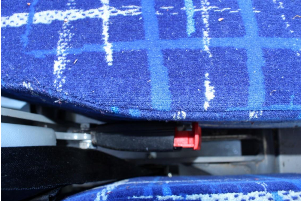
Photo #13: Defective seatbelt buckle for window seat
