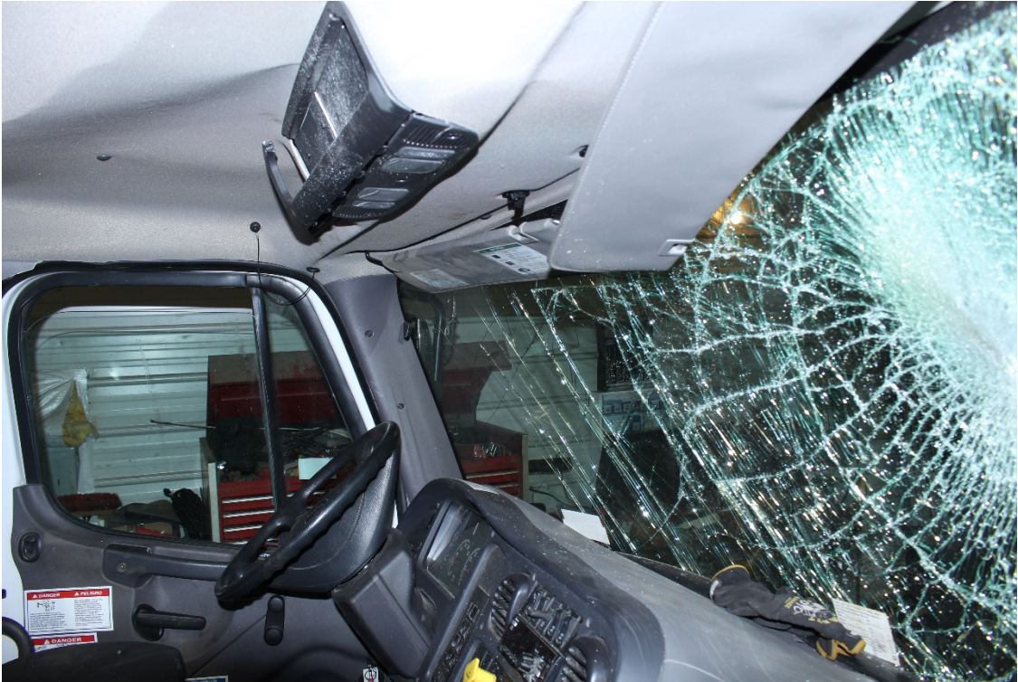
Photo #8: Interior view of trash truck cab and shattered front windshield
