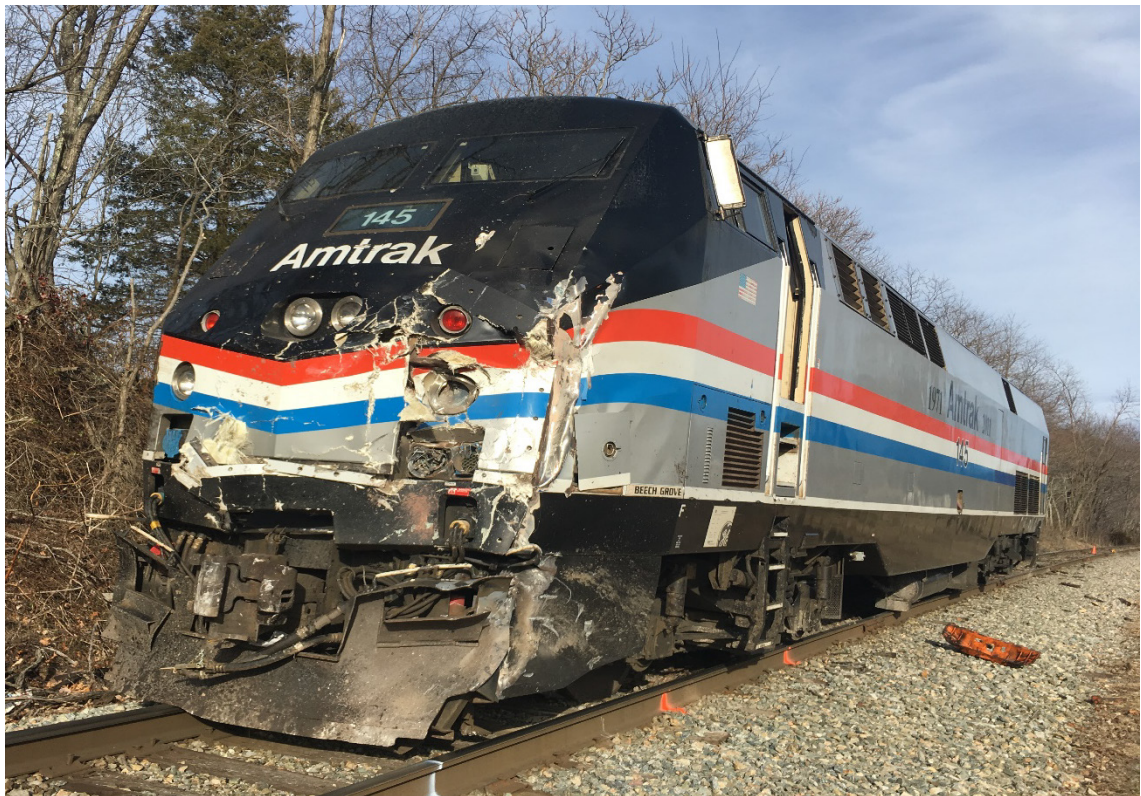
Photo #1: Exterior view of front of lead locomotive and damage caused by collision
