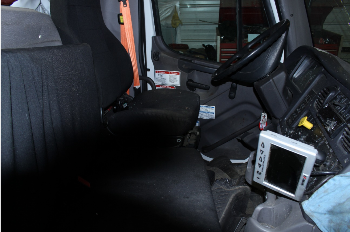
Photo #7: Interior view of trash truck cab, displaced seat and computer terminal
