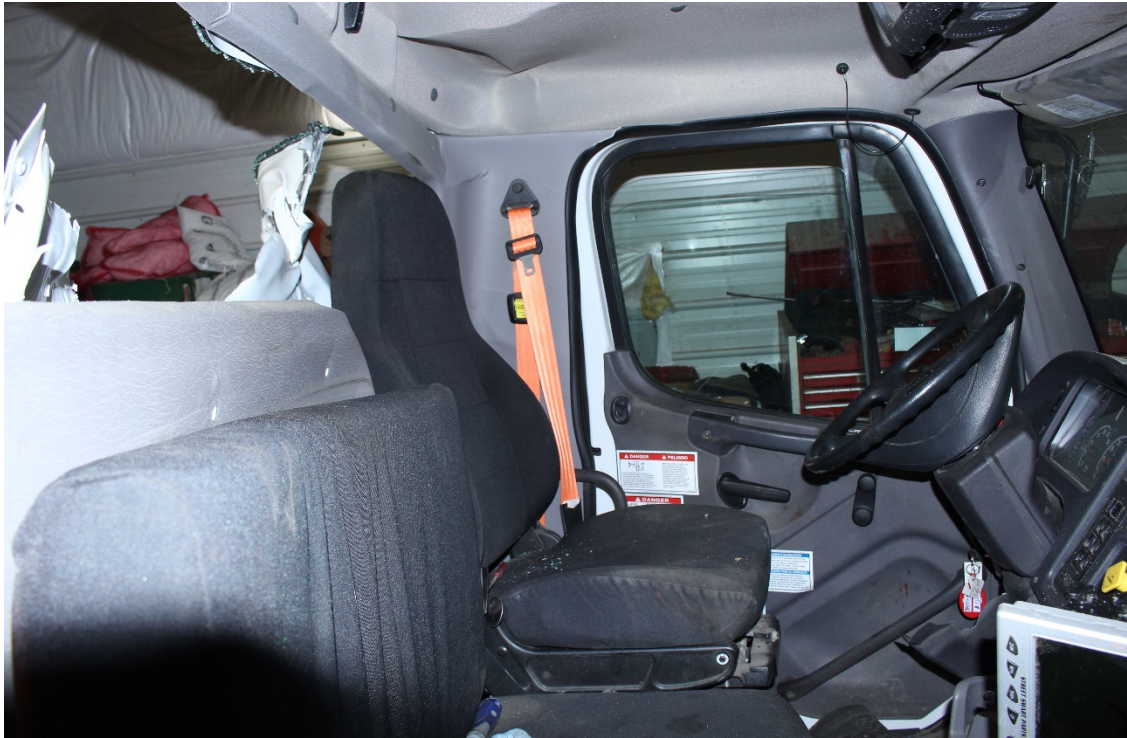
Photo #9: Interior view of trash truck cab and deformation of rear wall and bench seat
