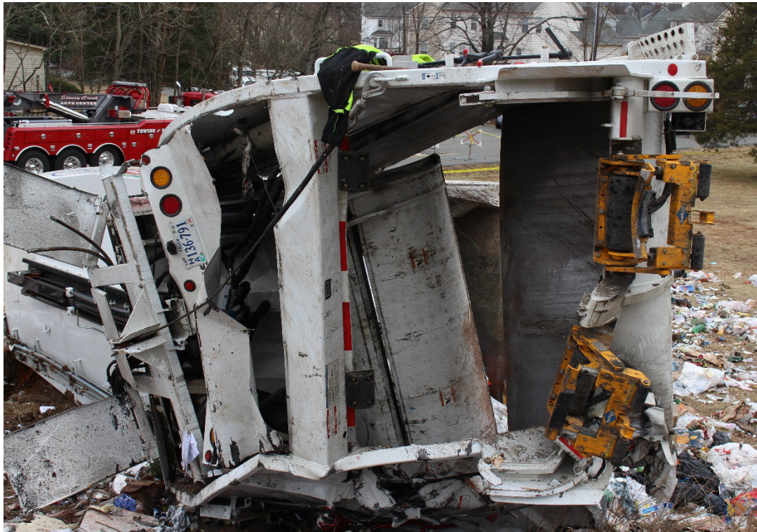
Photo #6: Rear view of detached trash truck hopper at final rest
