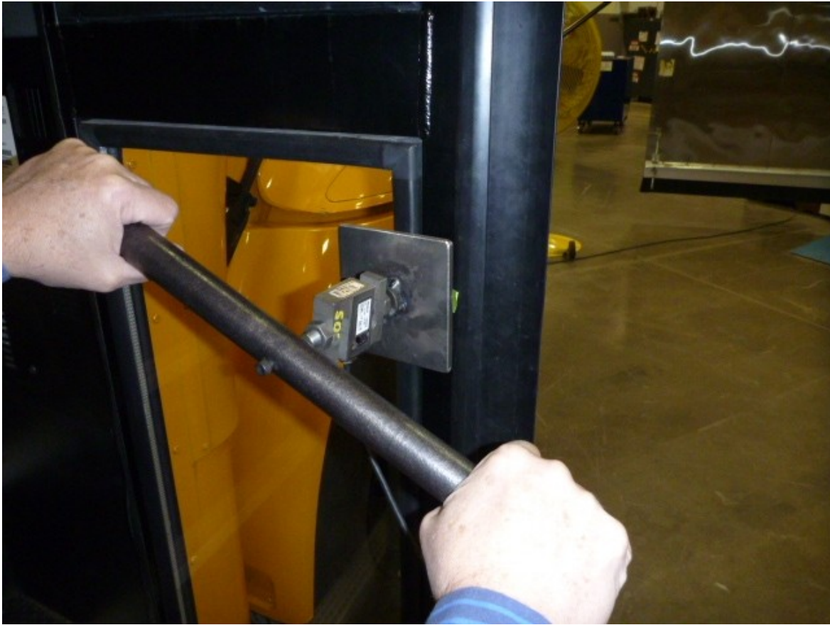
Figure 1: Force applied to open door at a height 36 in from floor lift
