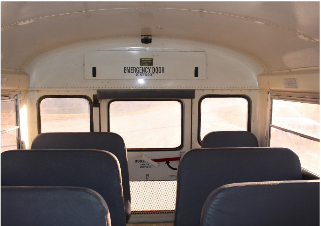
Photo #16: Close-up of rear emergency door and handle in exemplar school bus
