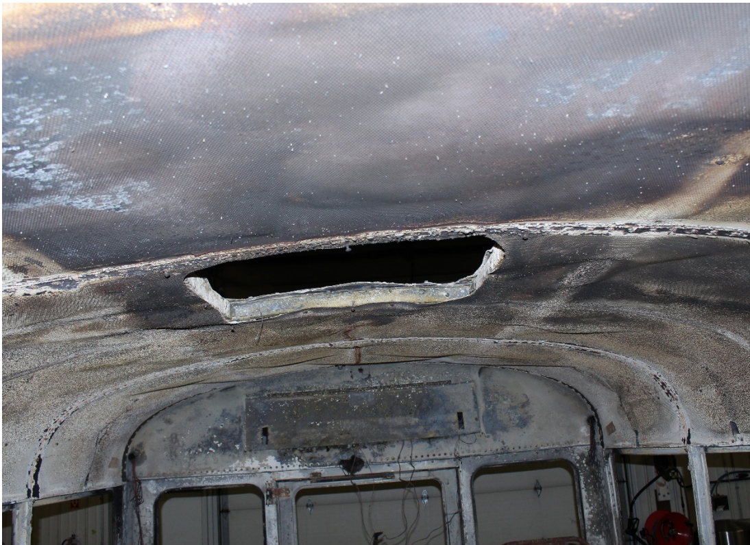
Photo #6: Interior close-up of rear roof hatch, missing cover and deformation to roof.
