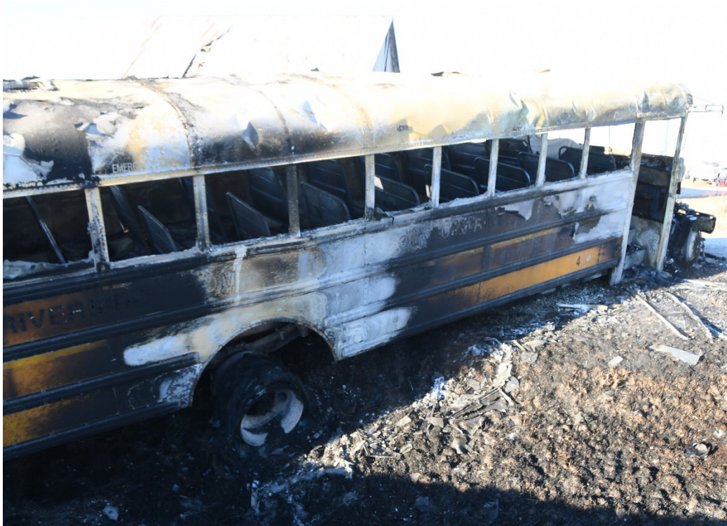
Photo #1: Exterior of school bus showing extensive fire damage at the scene
