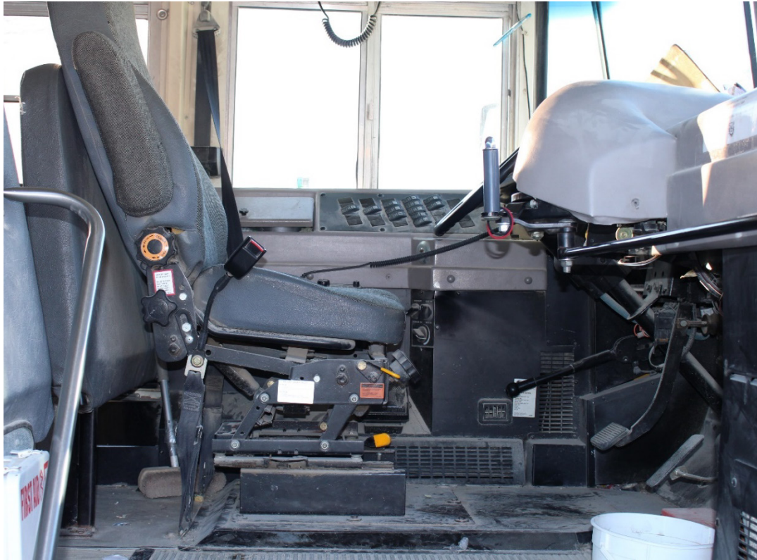
Photo # 13: Interior view of driver's area in exemplar school bus showing manual door release handle
