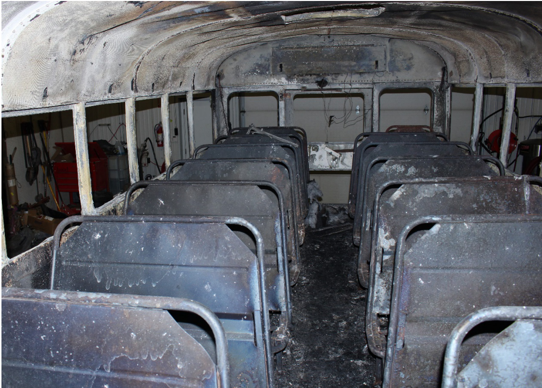
Photo #7: Interior view of the rear emergency door and fire damage to passenger compartment
