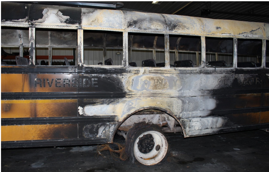
Photo #2: Left side exterior view of school bus showing extensive fire exposure.
