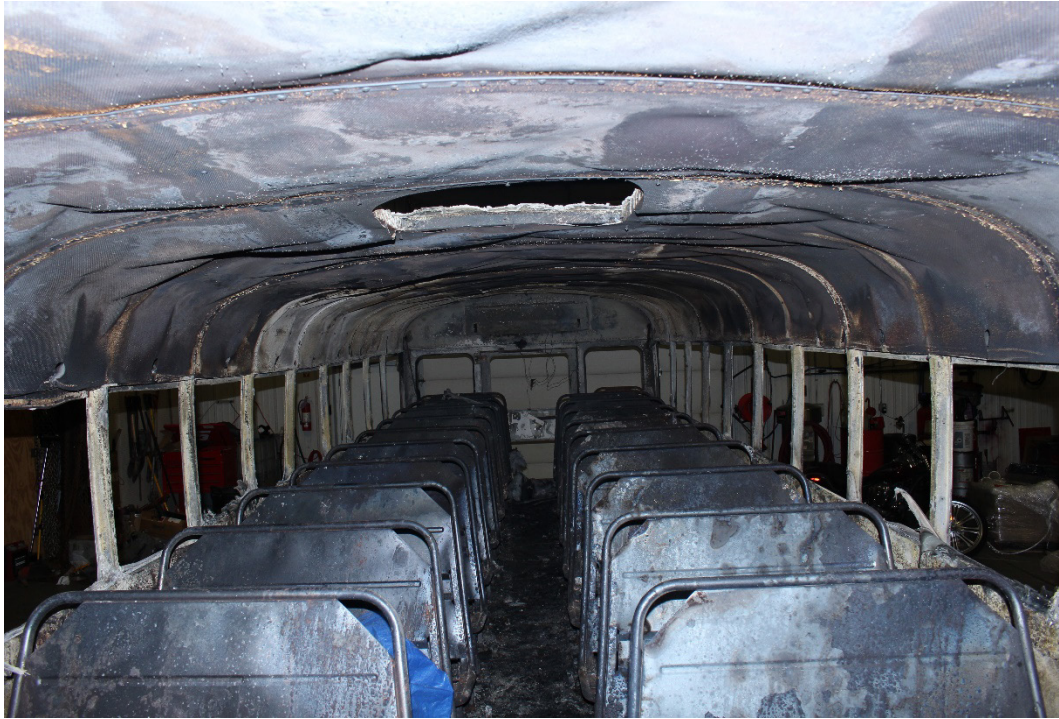
Photo #5: Interior of passenger compartment of school bus showing structural buckling
