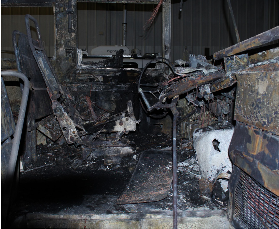
Photo #3: Front interior view of bus showing extensive fire damage at location of manual door release handle
