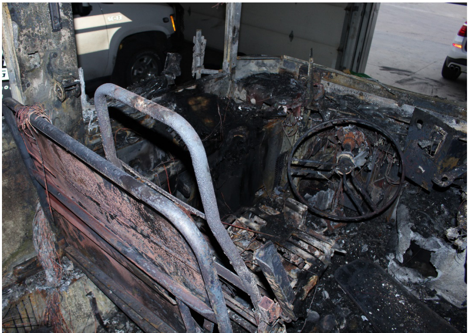
Photo #4: Interior close-up of driver's area showing extensive fire damage
