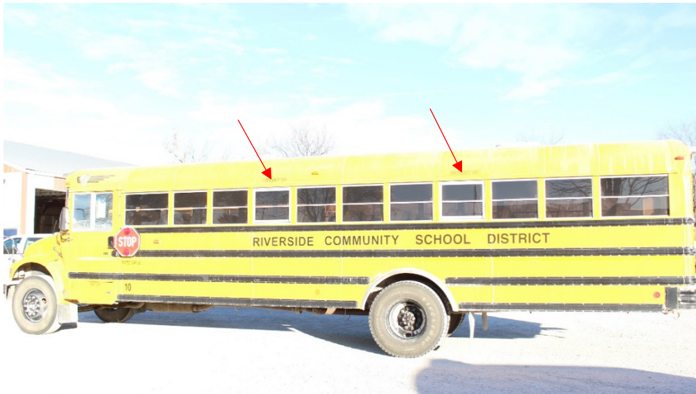
Photo #12: Exterior side view of exemplar school bus showing location of emergency windows
