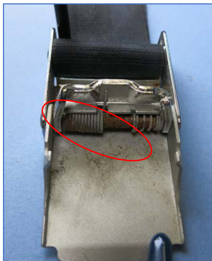
Figure 4 – Corrosion inside buckle lever.
