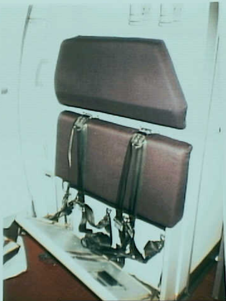
Survival Factors 6 - Photo 9. Forward flight attendant jumpseat (seat cushion removed).
