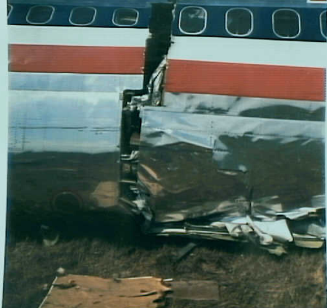
Survival Factors 6 - Photo 7. Cockpit damage, left side.
