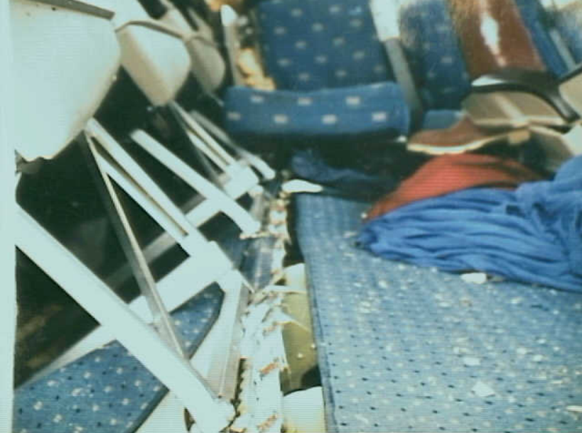
Survival Factors 6 - Photo 46. Seat legs, rows 24 - 26 (photo taken after wreckage moved to hangar).
