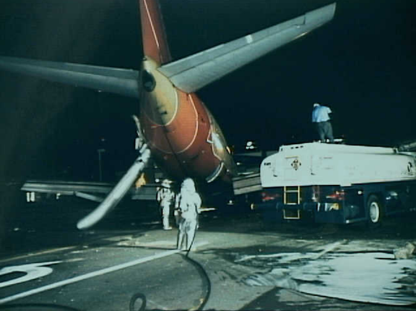
Survival Factors 6 - Photo 4. Escape slide at the aft, left exit.
