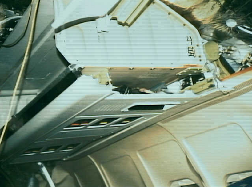
Survival Factors 6 - Photo 38. Interior damage, rows 13 and 14, left side.
