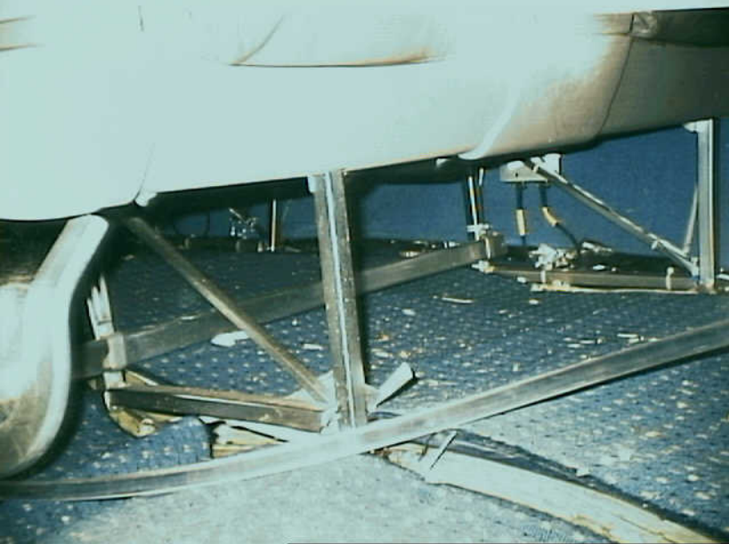
Survival Factors 6 - Photo 36. Interior damage, floor disruption at row 10/11.
