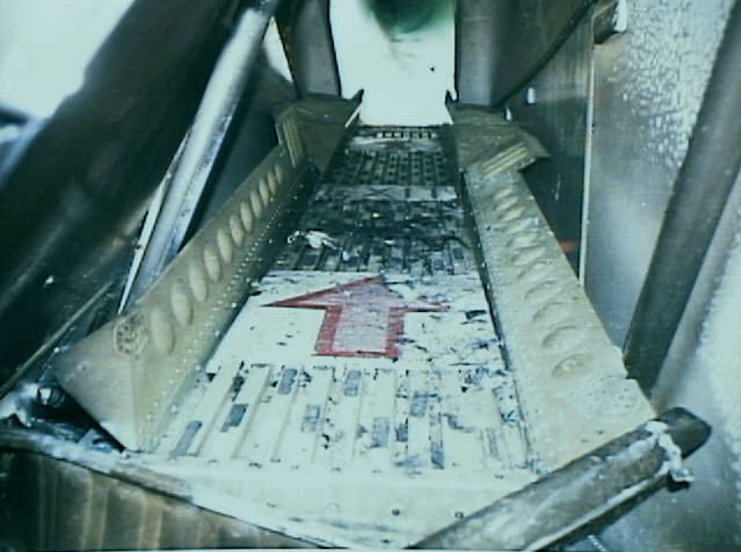
Survival Factors 6 - Photo 31. Interior damage, forward of row 7, looking aft
