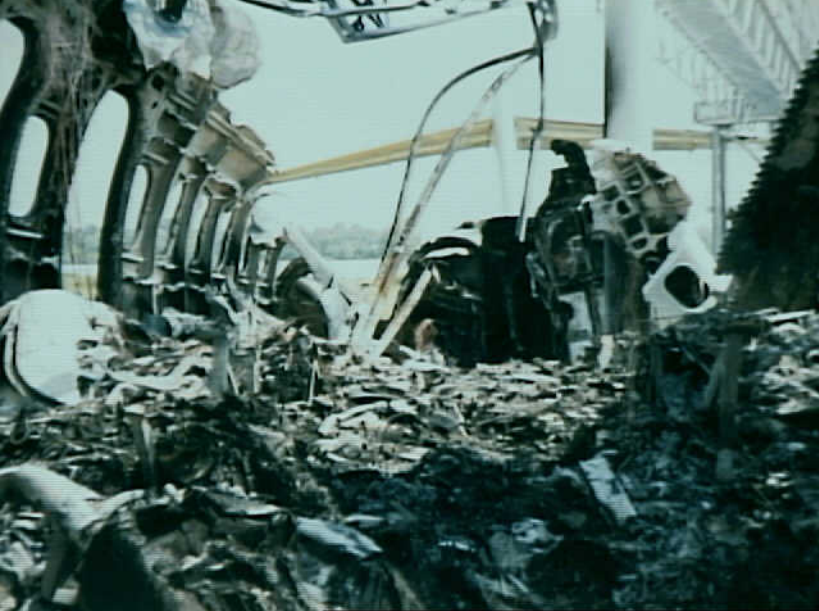
Survival Factors 6 - Photo 22. Fuselage break at row 18, looking forward.
