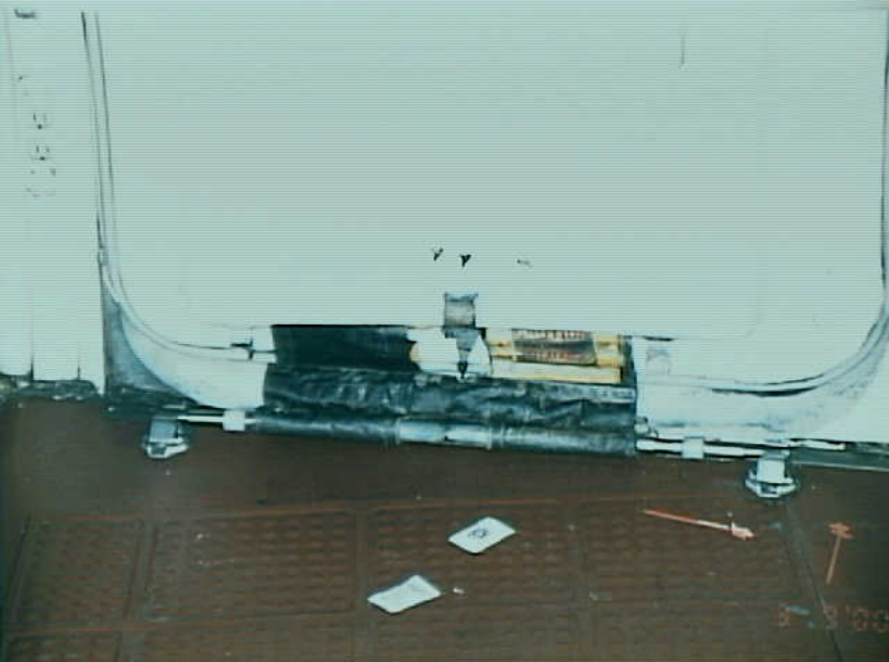
Survival Factors 6 - Photo 19. Girt bar, aft, right exit.
