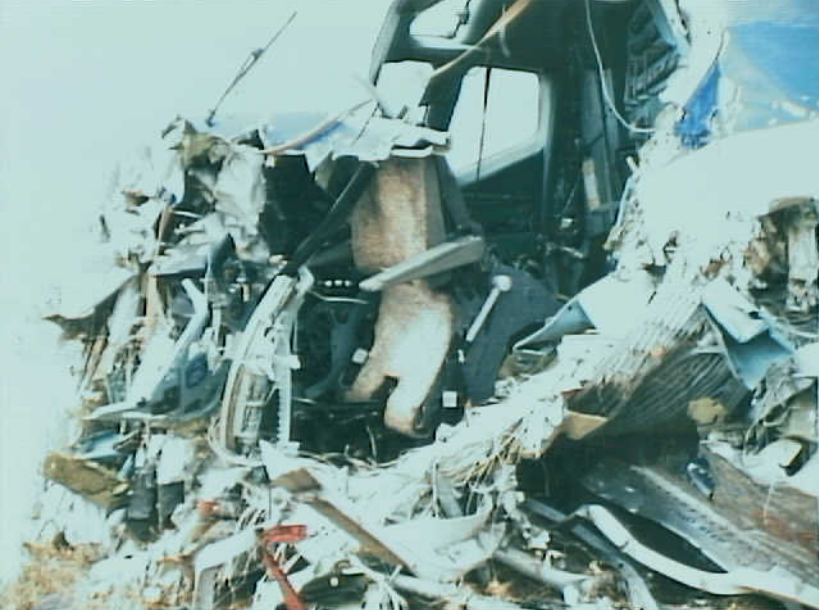
Survival Factors 6 - Photo 10. Exit 1R, forward service door.
