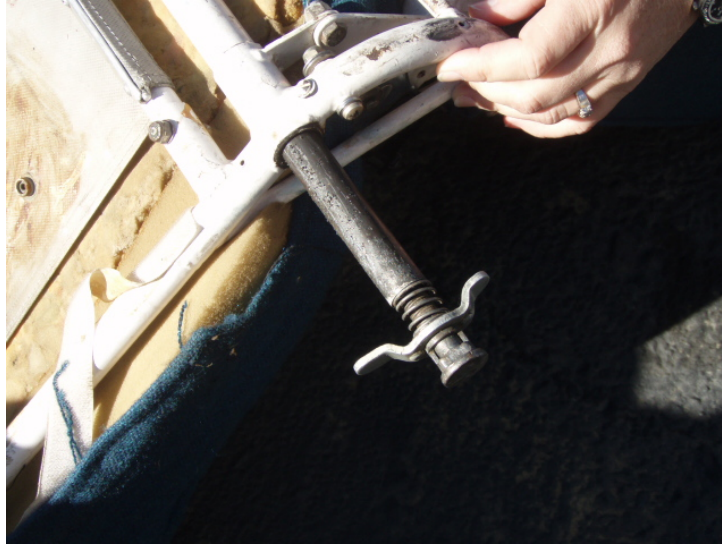
Figure 4. Photograph of a single pin hold down fitting
