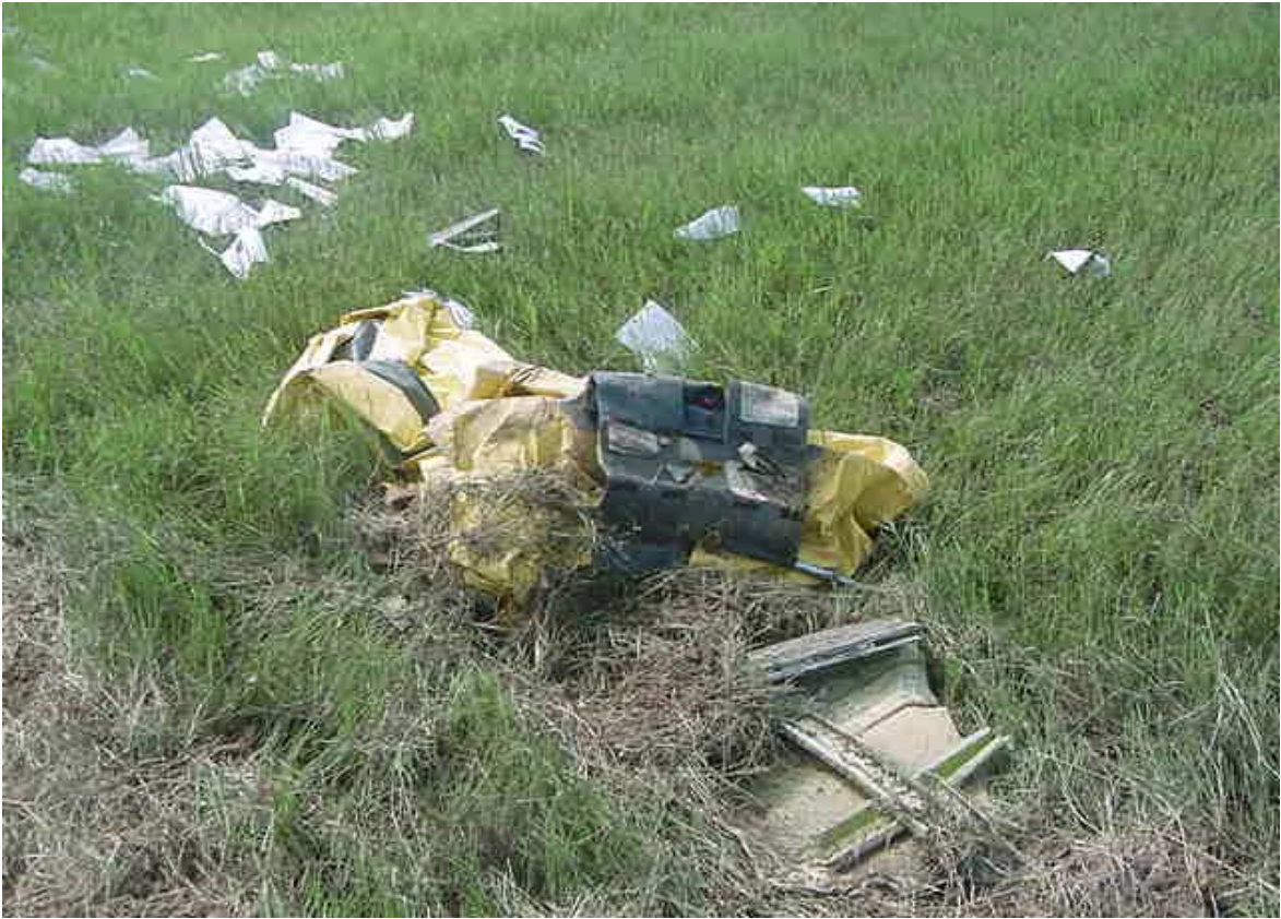
Photo 5: Evacuation slide from the 1L door, in the wreckage path.
