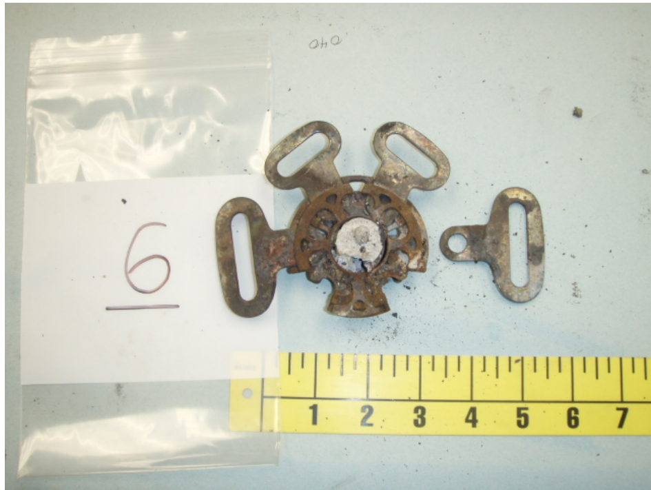
9. Photograph of the restraint cataloged as #6. Note: All latches engaged except the left (fixed) latch, which exhibited a shiny unscorched area where the latch would have engaged into the buckle.
