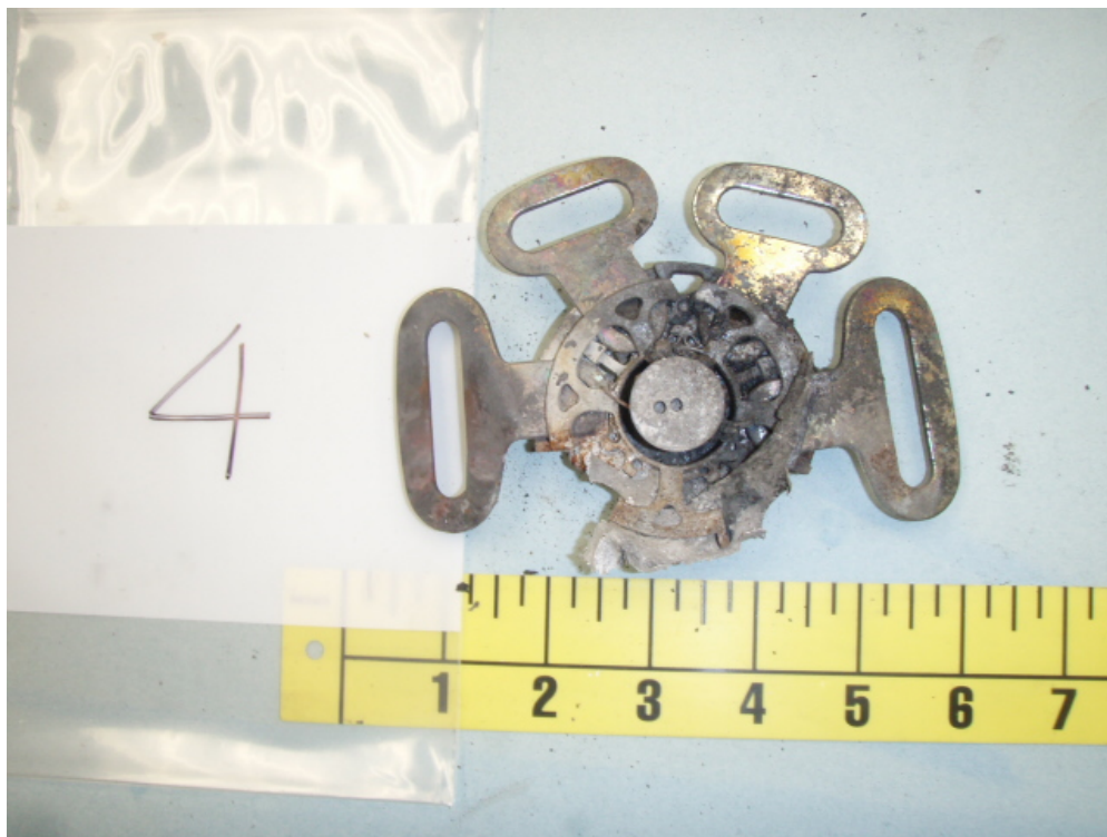
6. Photograph of the restraint cataloged as #4 buckle. Note: All latches are engaged.
