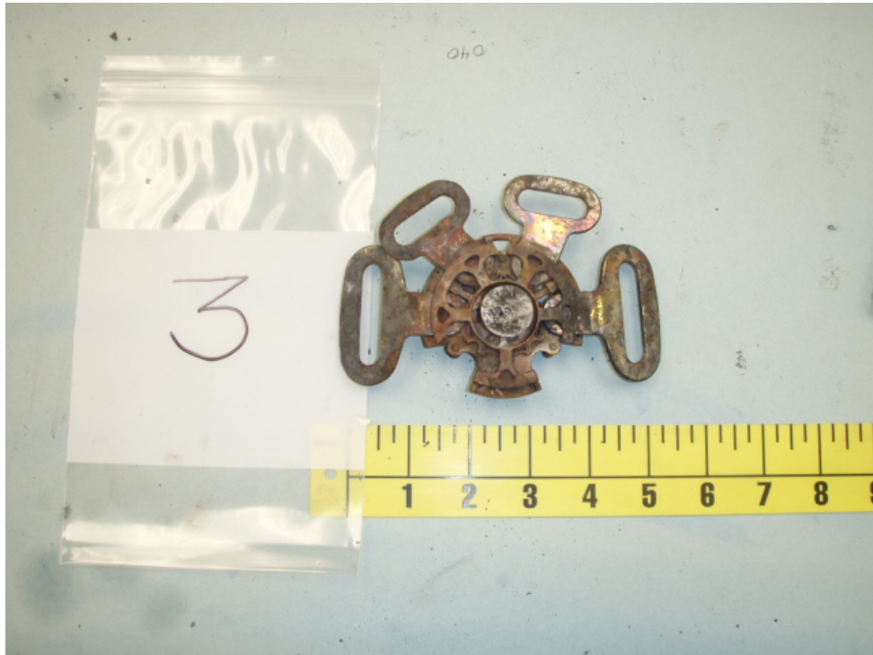
5. Photograph of the restraint cataloged as #3. Note: All latches are engaged.
