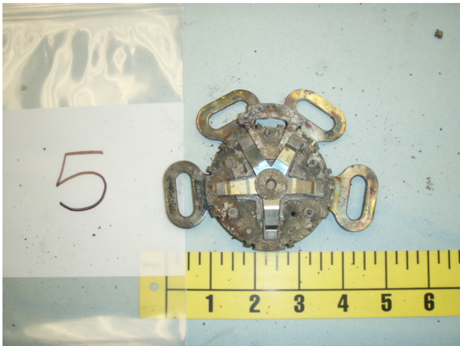
8. Photograph of a flight crewmember (Pacific Scientific) restraint cataloged as #5. Note: All latches were found engaged in the correct positions.
