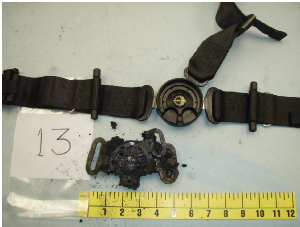
16. View of the restraint cataloged as #13. Note: Right shoulder harness is unlatched, and the left shoulder harness is latched 180 degrees opposite its correct engagement position.
