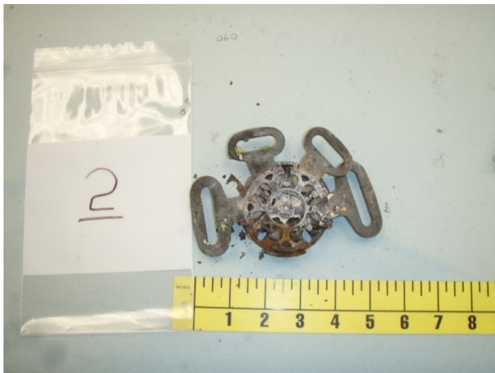
4. Photograph of the restraint cataloged as #2. Note: All latches are engaged.
