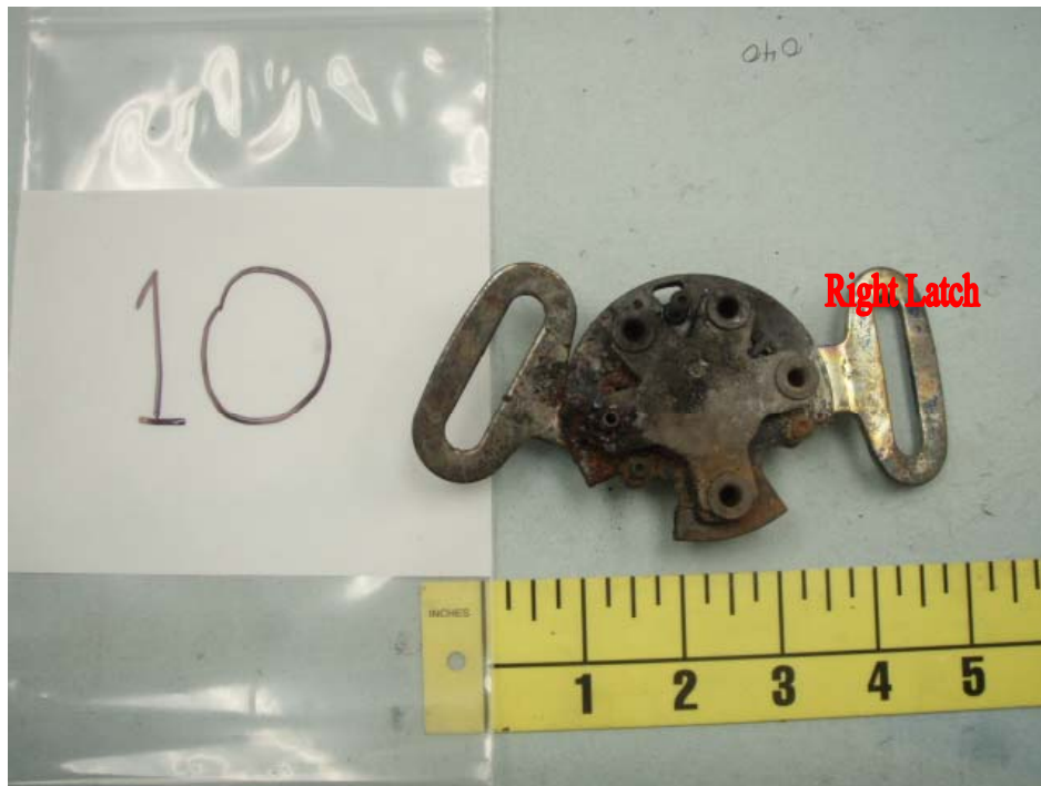
13. View of the restraint cataloged as #10. Note: The buckle is face down, and its right lap latch is latched 180 degrees opposite its correct engagement position.
