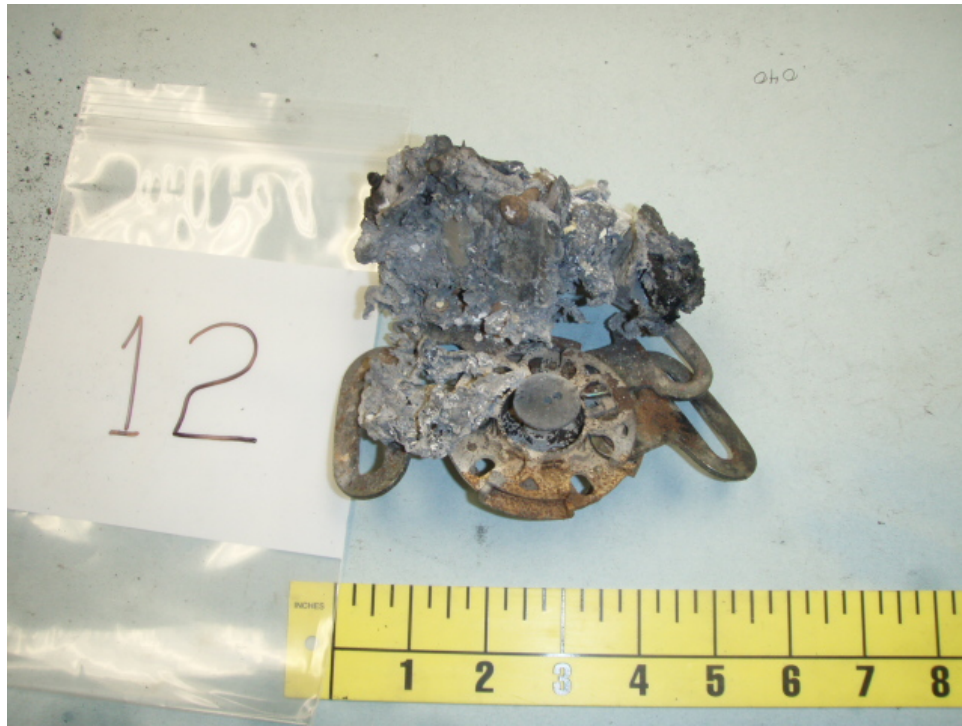
15. Photograph of buckle cataloged as #12. Note: All latches engaged in correct positions.
