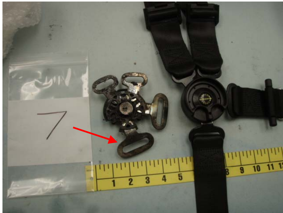
10. Photograph of restraint cataloged as restraint #7. Note: Red arrow points to the right lap restraint latched in the crotch engagement position.
