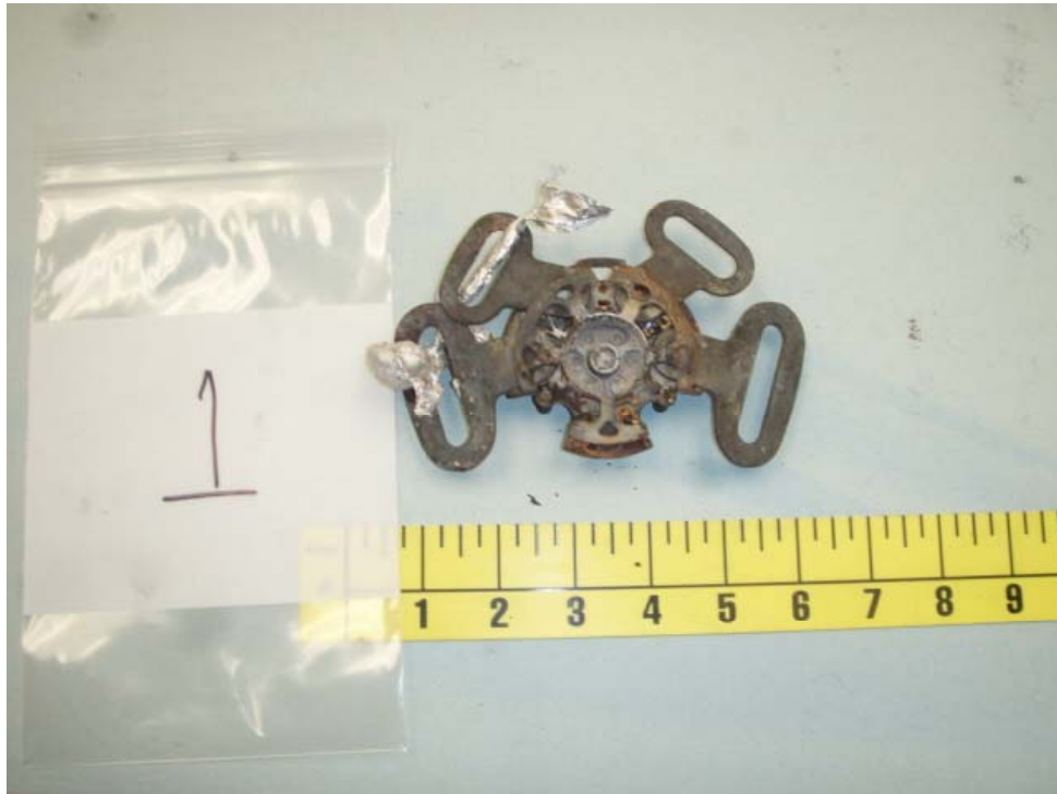
3. Photograph of the restraint cataloged as #1. Note: All latches are engaged.
