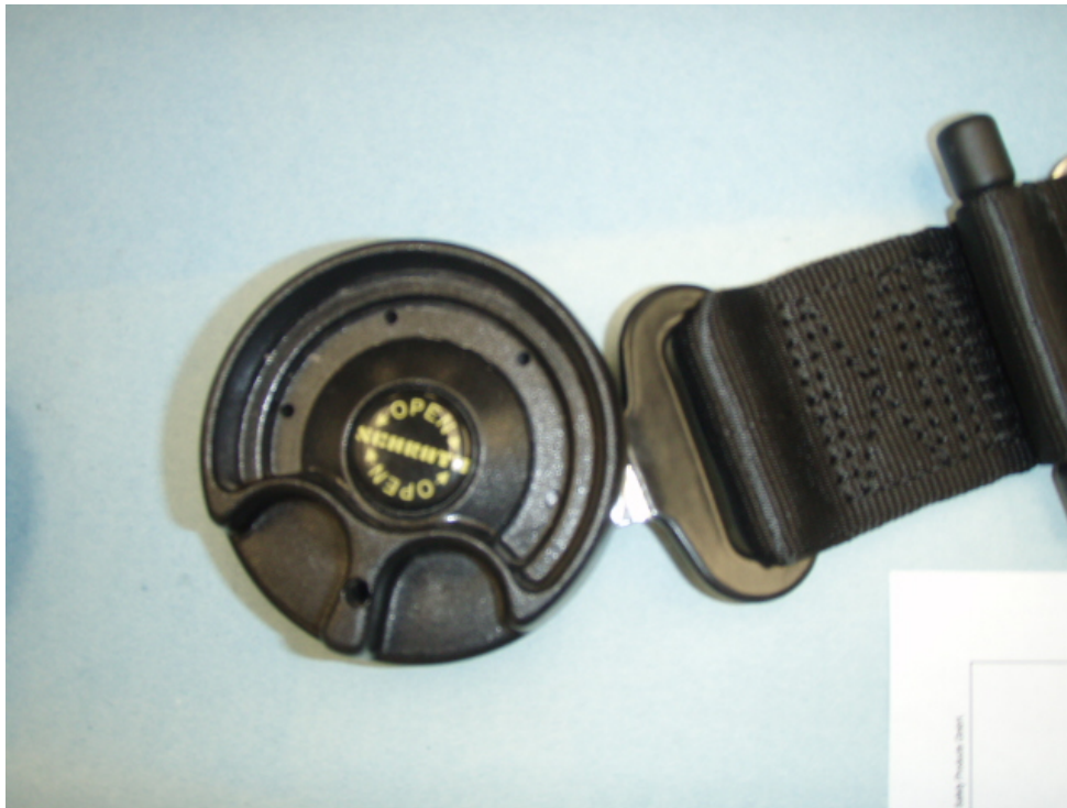
1. Photograph of a Schroth (SL 12.5) restraint unbuckled with the (occupant's left) fixed restraint installed in the buckle.
