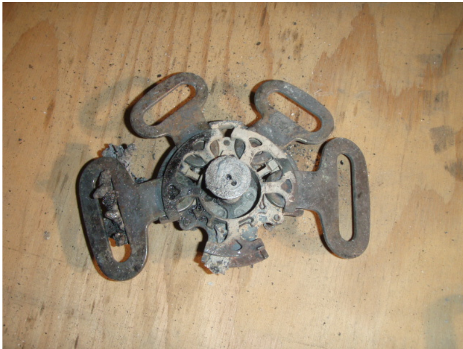
18. Photo of the restraint cataloged as #15 found during the October 28, 2008 wreckage exam. The buckle's lap and shoulder restraints are latched.
