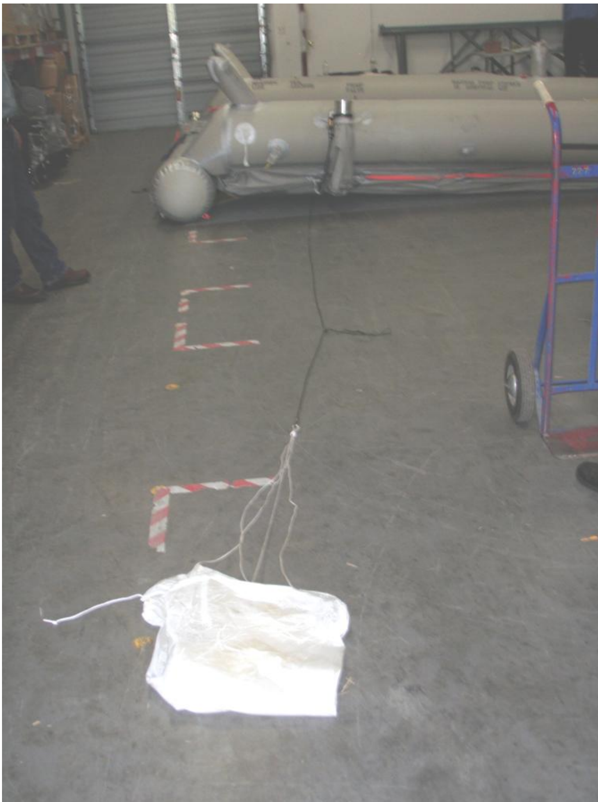
8. Photograph of the 1R slide/raft with the sea anchor removed from the aspirator Note: The slide/raft lower tube partially deflated.
