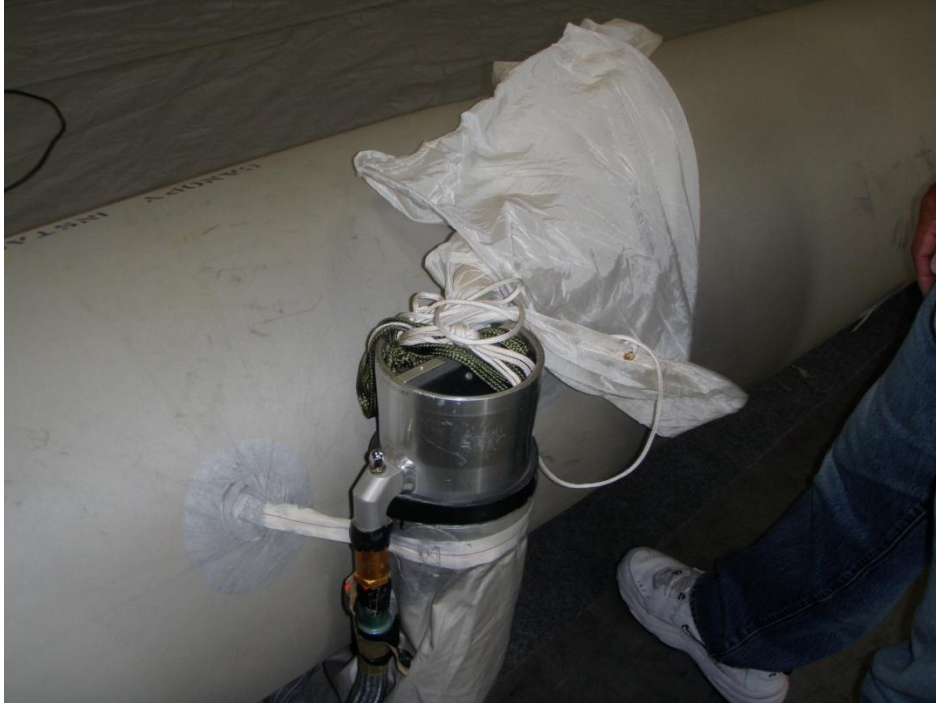
4. Close up view of the sea anchor and sea anchor line ingested in 1R aft aspirator.
