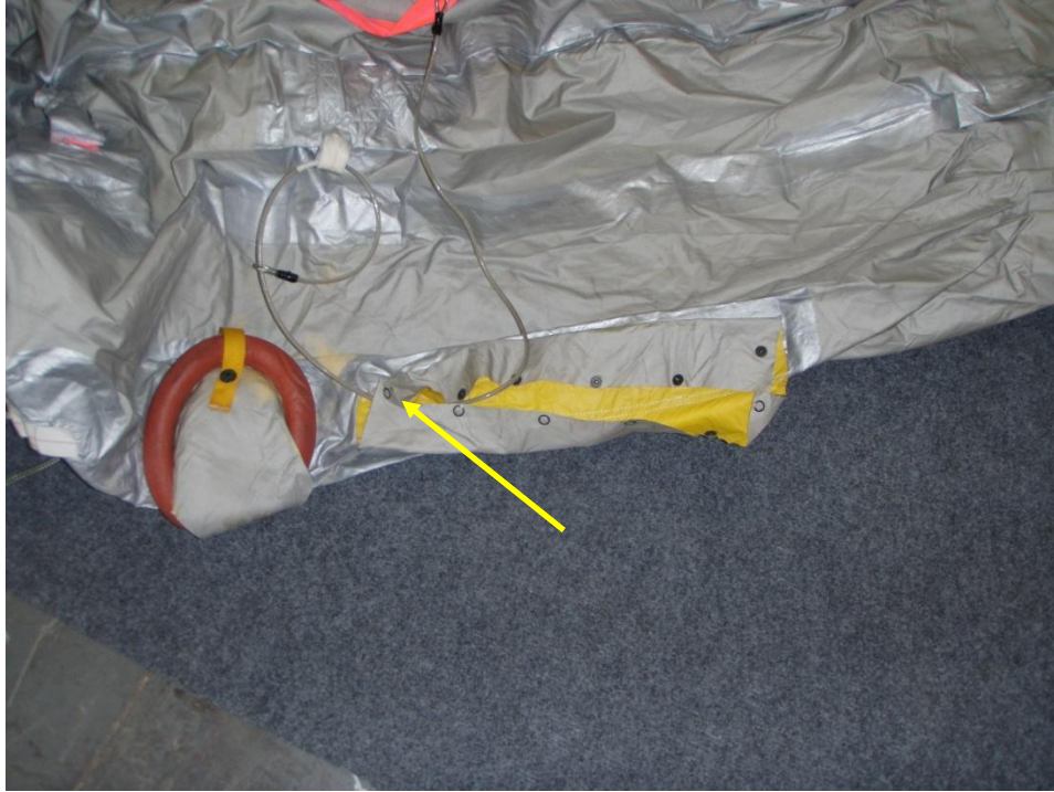
2. Photograph showing the sea anchor pouch as it was found with the stainless steel cable routed through the sill end of the pouch.
