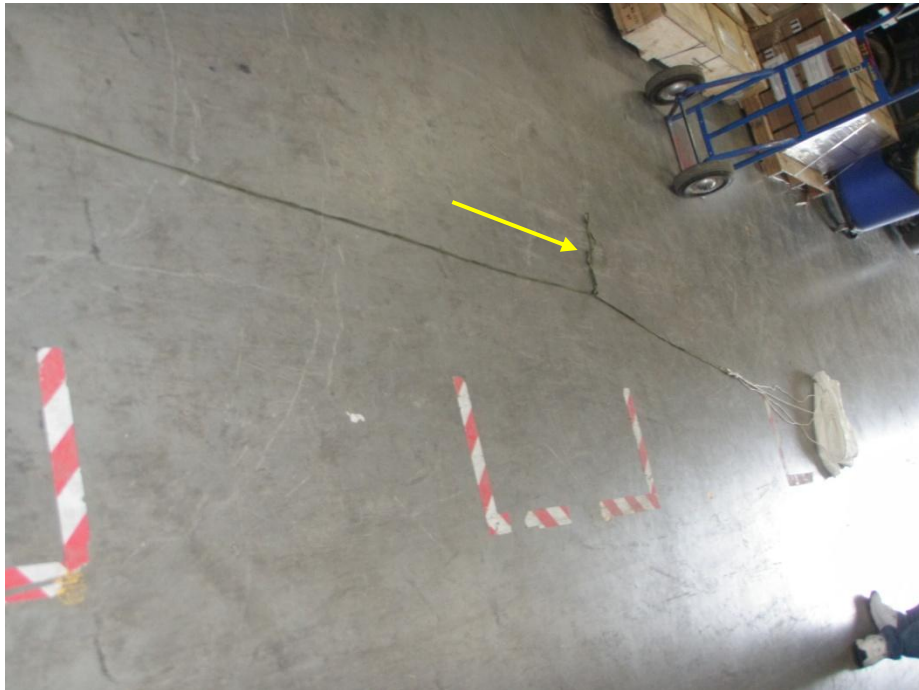
5. Photograph of the sea anchor and sea anchor line stretched out on the shop floor. Note: The yellow arrow points to the knot in the sea anchor line.
