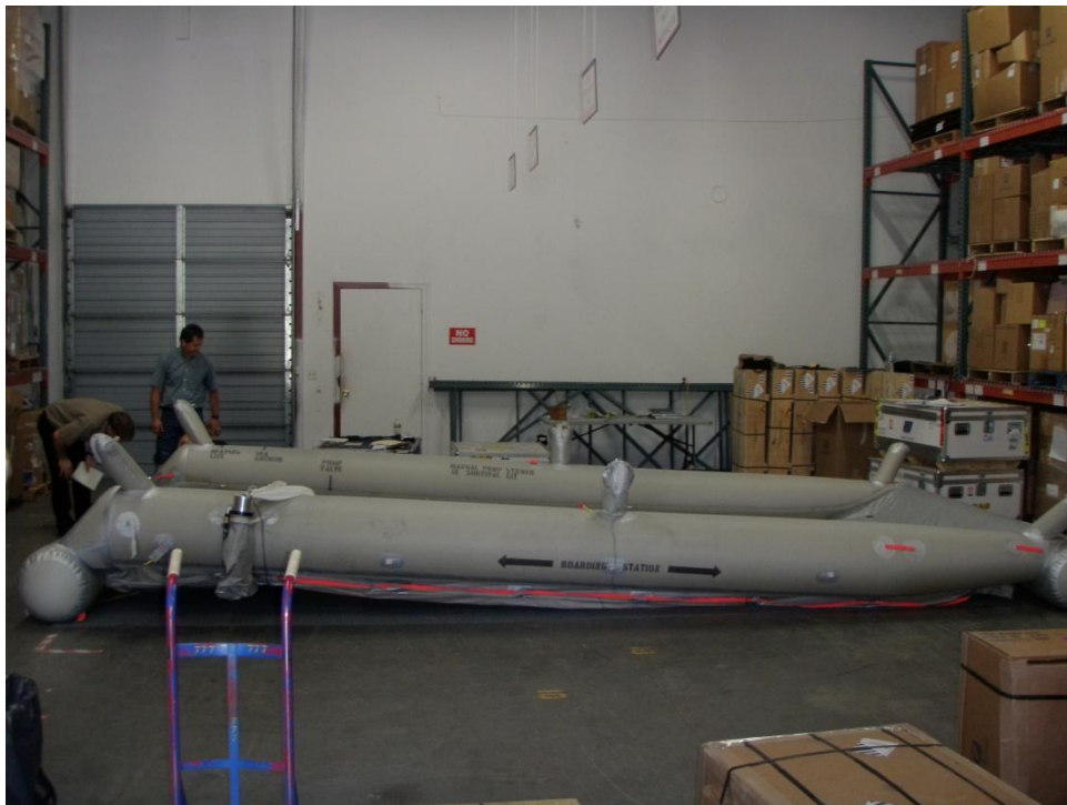
7. Photograph of the 1R slide/raft inflated with the sea anchor ingested in the aft aspirator.
