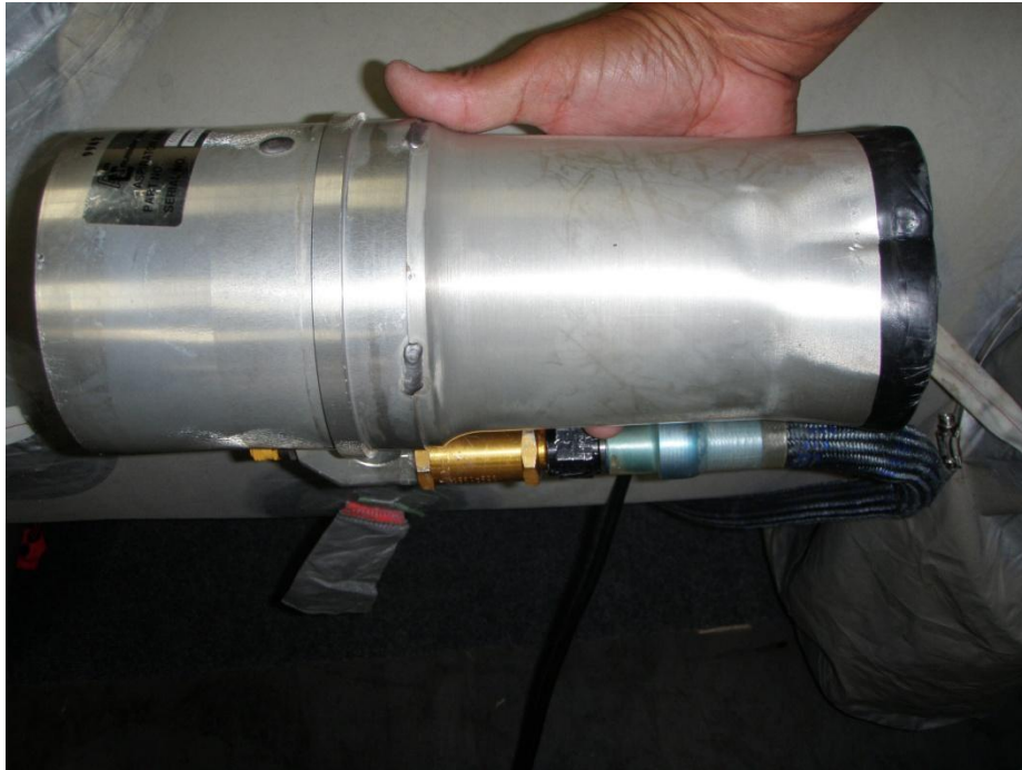
11. Side view of the disassembled forward aspirator chamber Note: The damaged and dented chamber.
