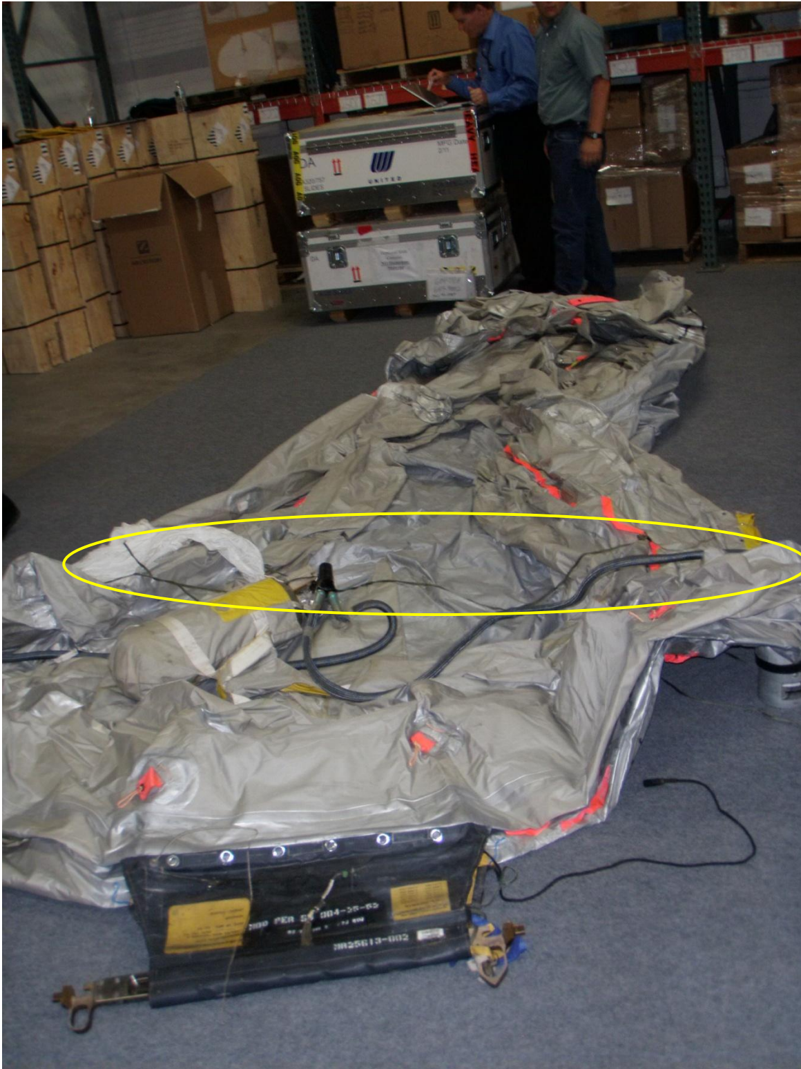
1. Photograph of inverted 1R slide/raft (bottom facing up) Note: Yellow oval shows the thin sea anchor line between the pouch and aft aspirator.
