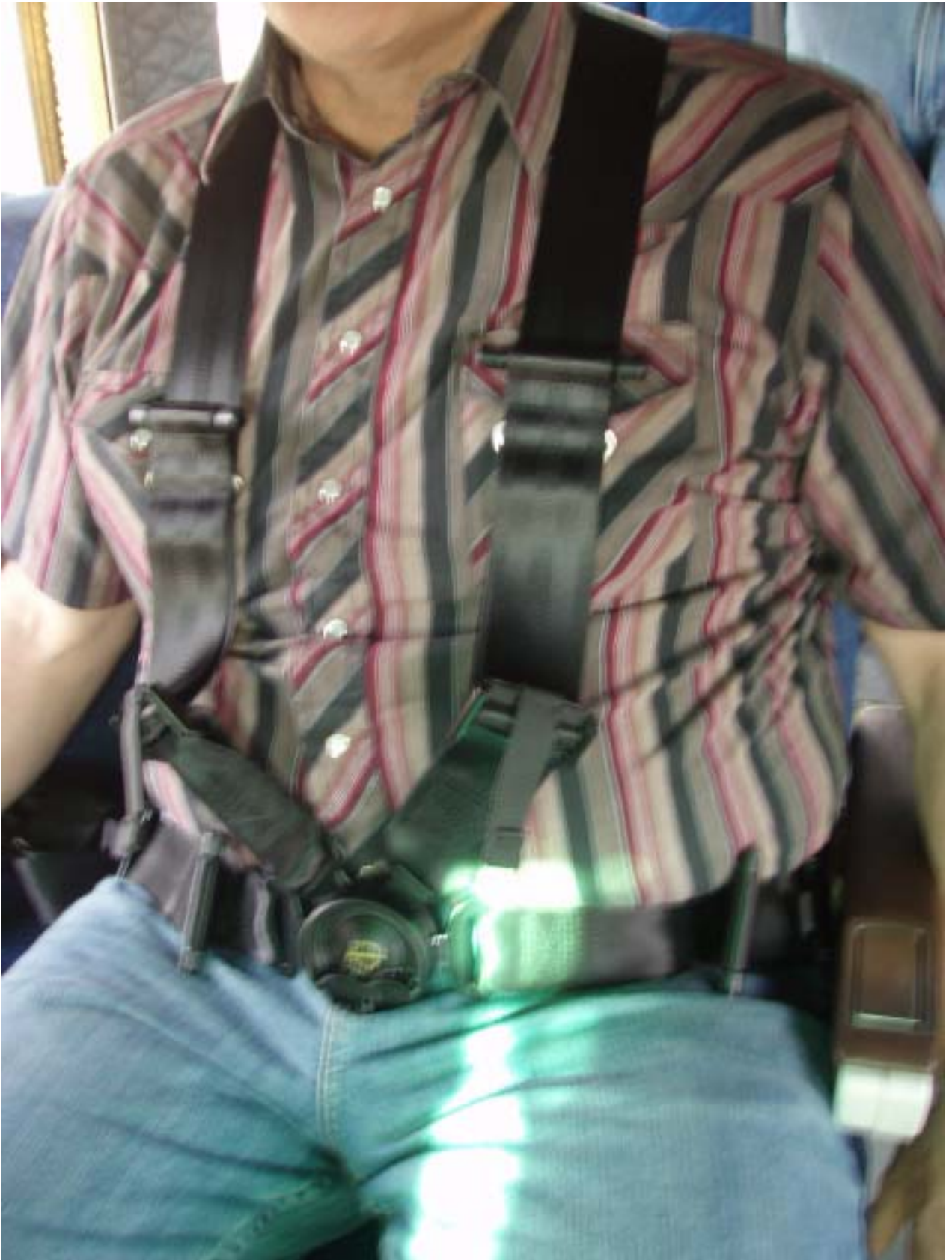
11. View of a buckled 4-point Schroth restraint (like the restraints installed in N612AZ.)
