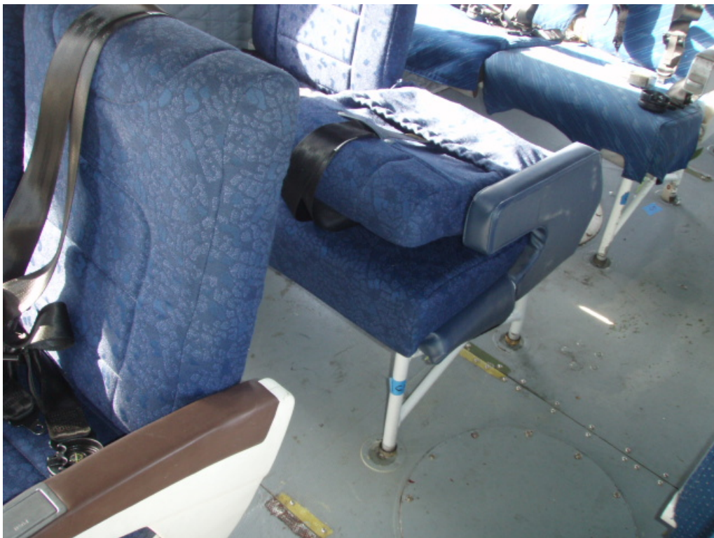
5. View of the inboard double seat back folded forward. Note: There was no mechanical stop to retain the seatback in the upright position.
