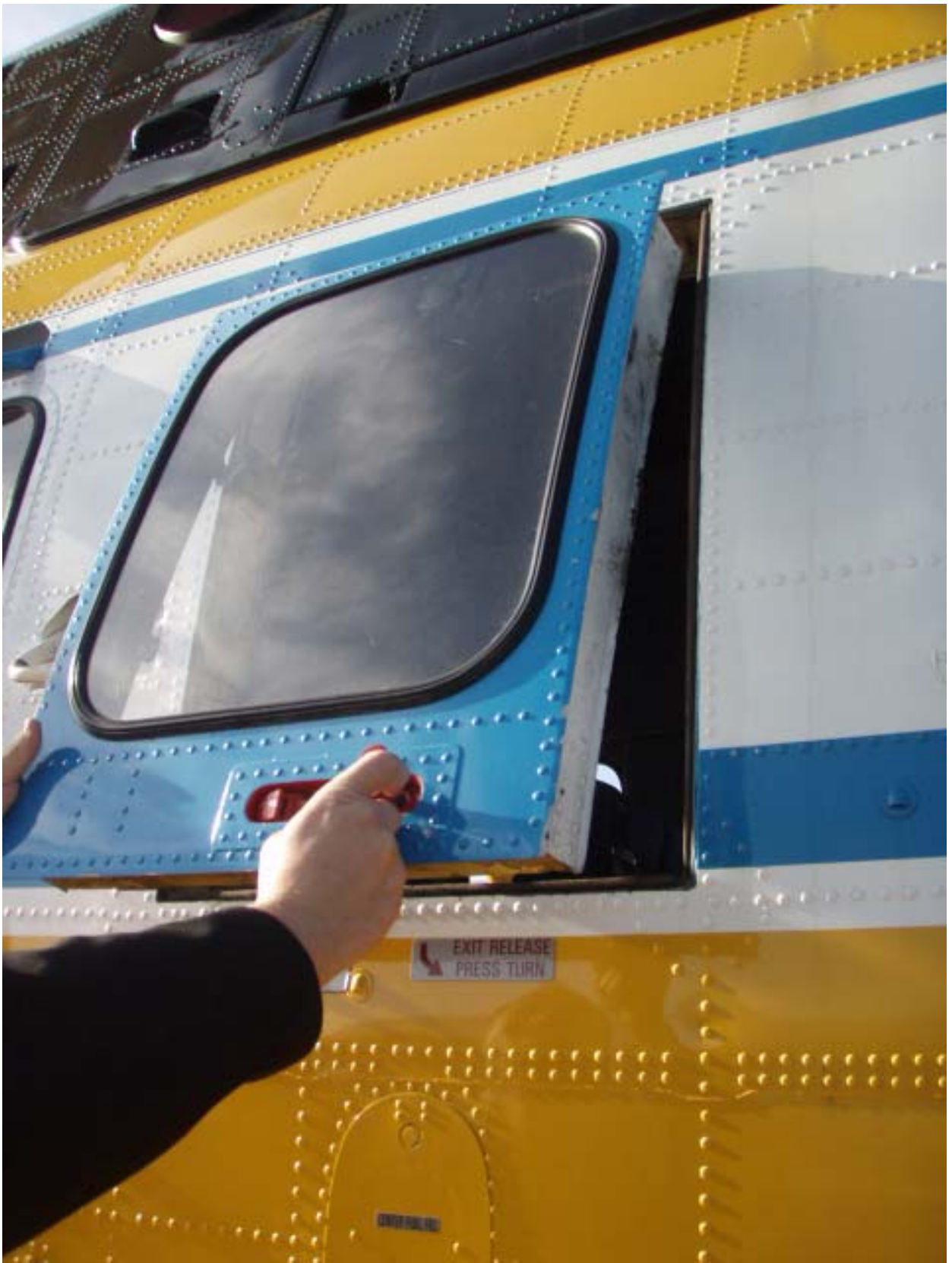
3. View of an emergency exit hatch being removed from N61NH.
