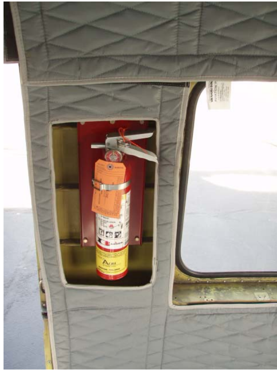
13. View of one of the two fire extinguishers in the S-61N helicopter. Note: Normally mounted in the aft left cabin next to the emergency exit hatch.
