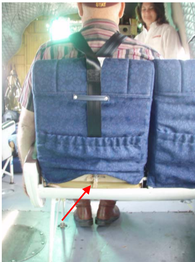
10. View of the rear of an outboard double seat. Note: Red arrow points to the shoulder restraint attachment to the seat crosstube.
