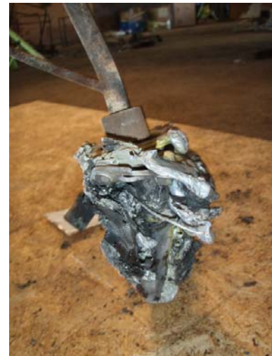
9. Close up of the fuel probe that melted to the aft seat leg, revealing that the double seat was from row 4 seats C and D on the right side of the cabin.
