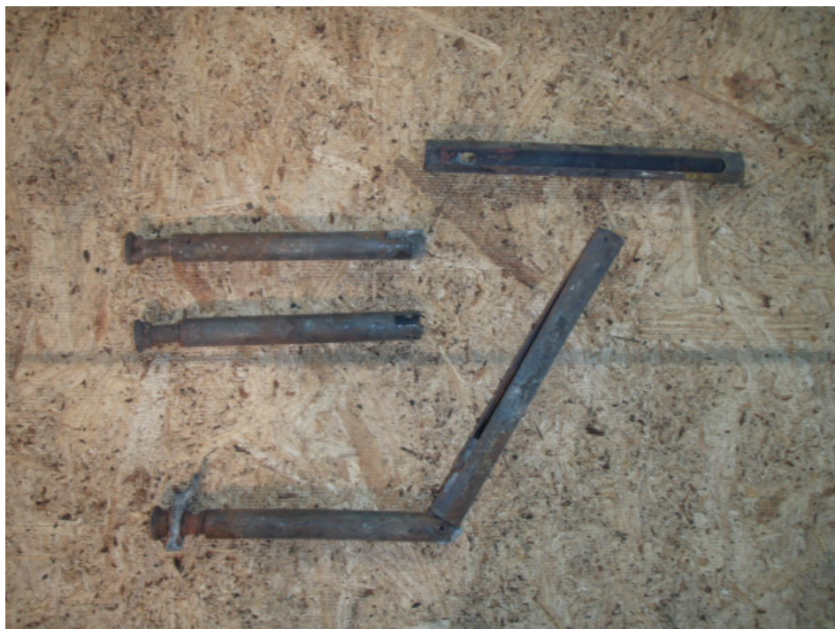
16. Photograph of single pin hold down fittings that were found in the wreckage.
