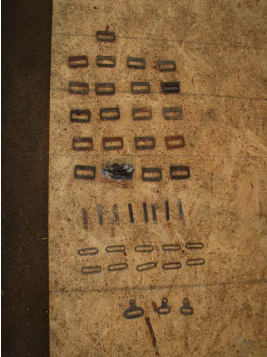
17. View of restraint steel hardware pieces that were found in the wreckage. Note: One lap-latch fitting and 2 shoulder restraint fittings are shown at the bottom of this photograph.
