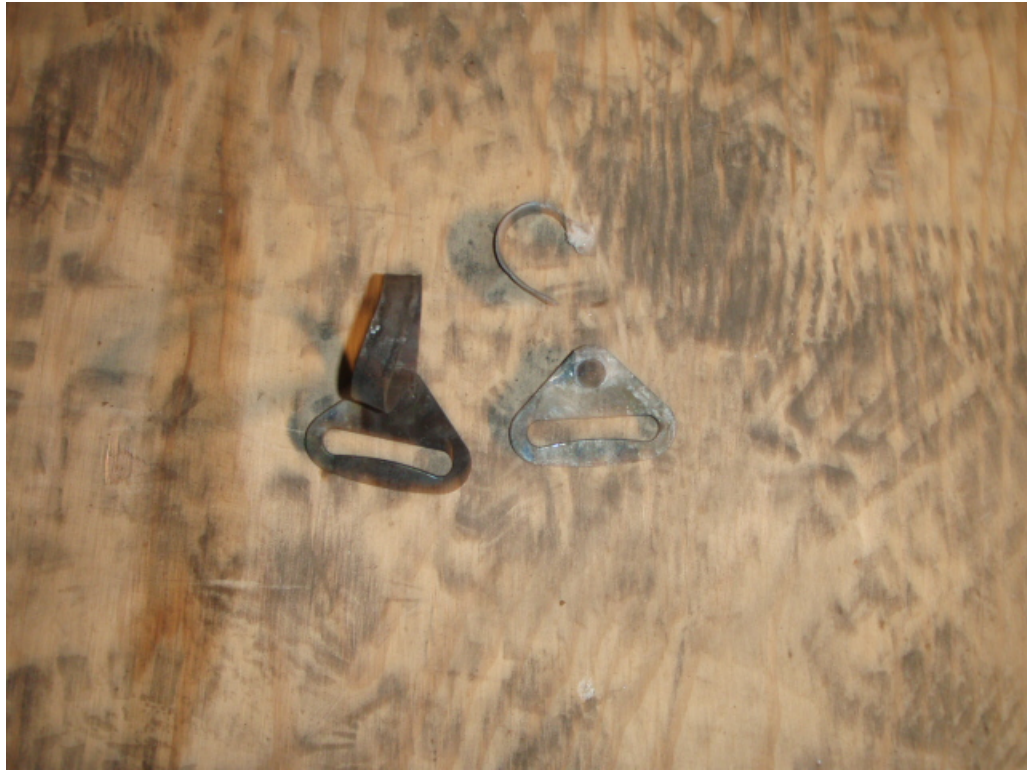
18. View of two shoulder restraint end fittings. The end fitting on the right became separated from the aidel clamp.
