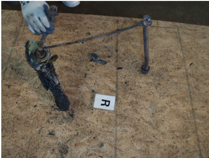
8. View of the seat legs that had separated from the seat and were cataloged as R above.
