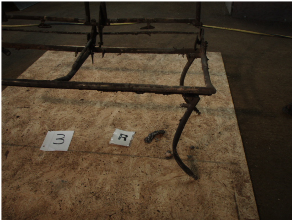
10. Photograph of the 3 rd double seat found in the wreckage. Note: The inboard seat legs exhibited compression bending and both hold down stud fittings separated from the seat legs.
