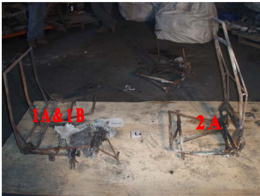
12. Photograph showing the aft facing double seat and a single high back single seat (for seat positions 1A and B and 2A.)
