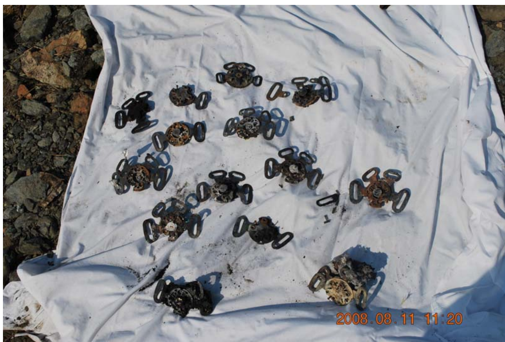
5. Photograph of the charred remains of restraint buckles removed from the wreckage.
