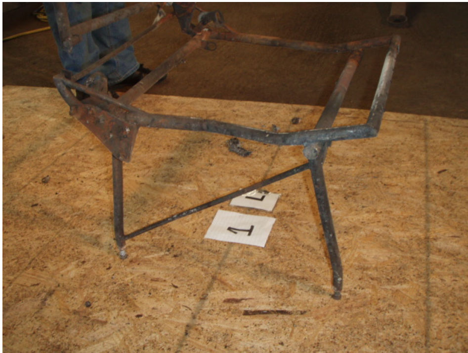
13. View of the inboard seat legs from a forward facing single seat. Note: The single stud hold-down fittings separated from the seat legs.
