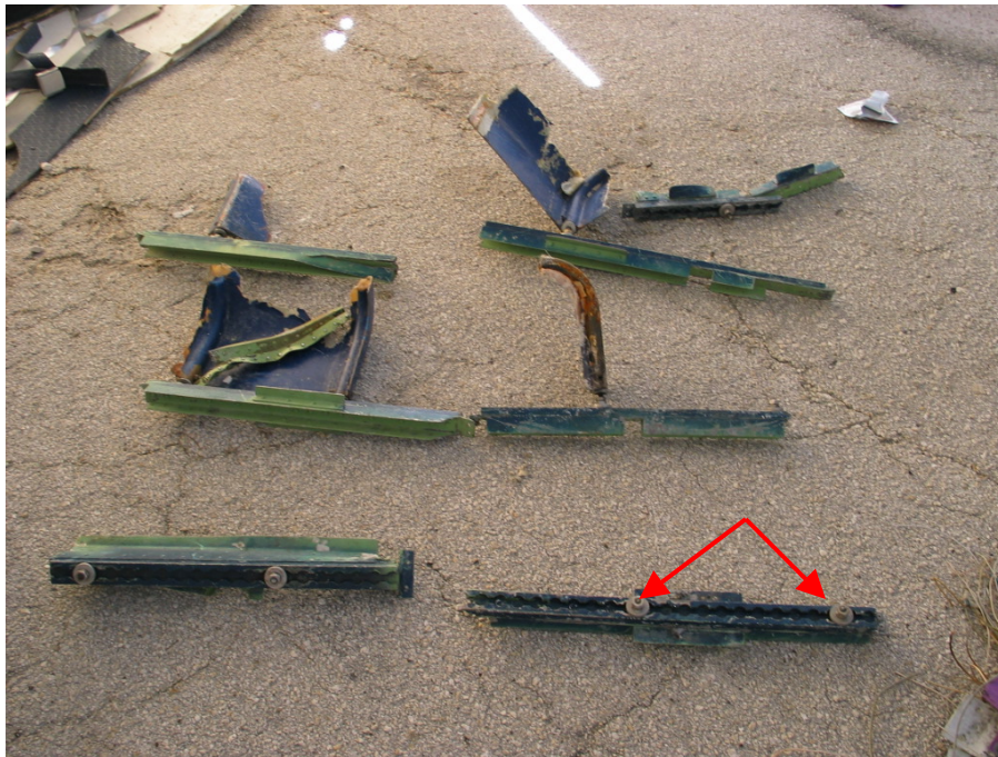
10. View of the 7 sections of fractured seat track that contained fractured seat legs or seat attach fittings in the seat tracks. Note: red arrows point to the attach fittings in the seat tracks.
