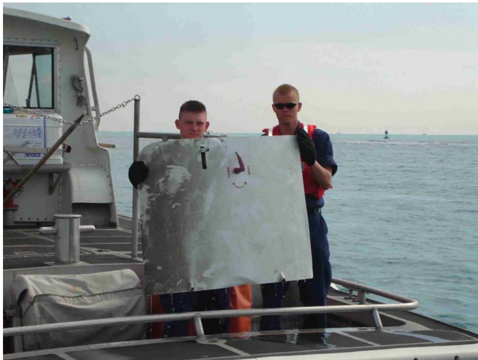
13. View of N2969's main cabin door after being recovered from Government Cut. Note: The door's handle was found in the latched position.
