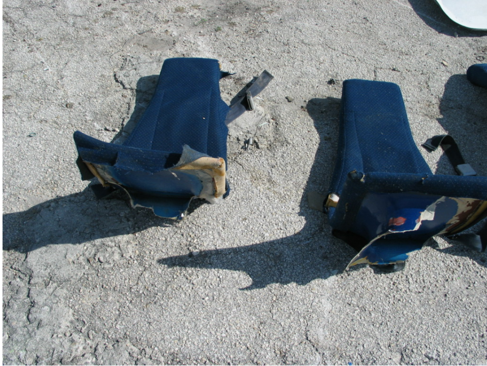
7. View of two passenger seat backs from N2969 that were found intact.
