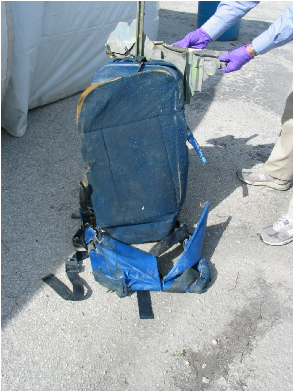
11. View of the Captain's seat from N2969. Note: Its seat back remained attached to the cockpit bulkhead.
