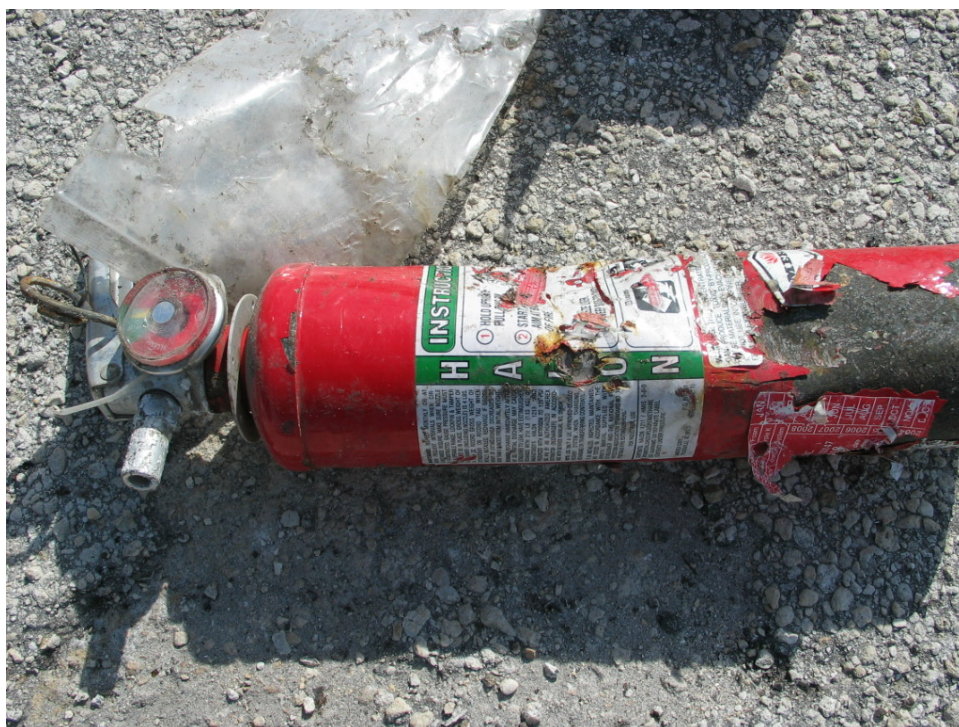
6. View of one of the Halon class C fire extinguishers that was recovered from Government Cut. Note: its gage was found in the charged position.
