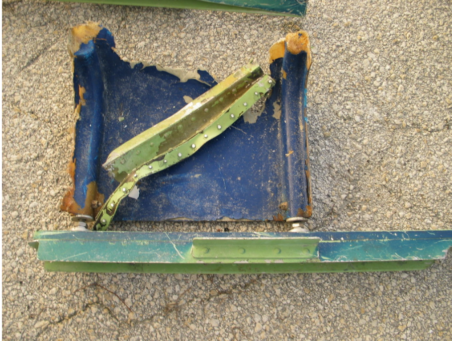
9. View of a passenger seat bottom from N2969, found installed in a fractured section of seat track
