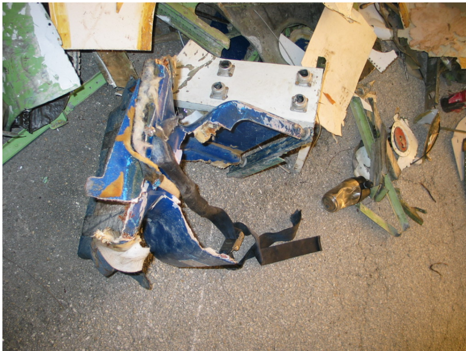
8. View of a fractured passenger seat bottom from N2969.
