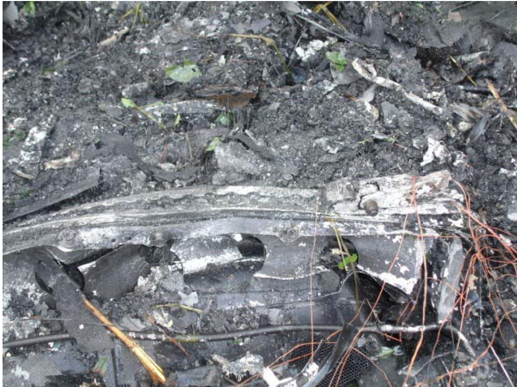
Photo 22. A section of floor track with a fractured aft seat attachment fitting
