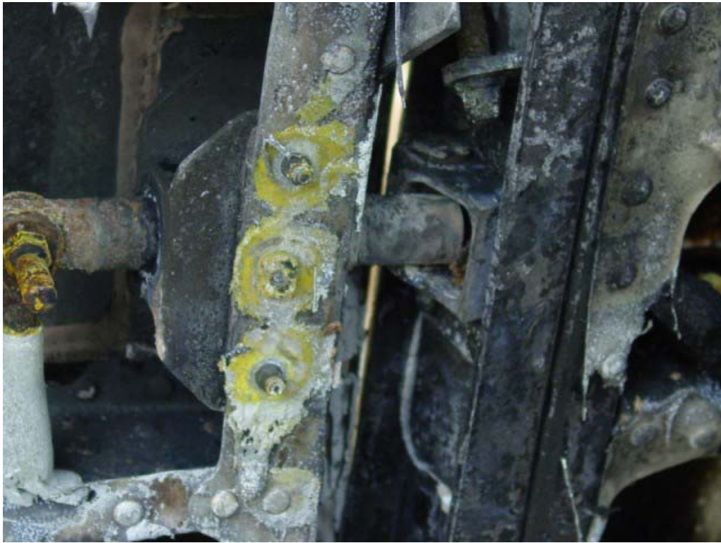
Photo 15. One of the main cabin door's extended forward lock pins
