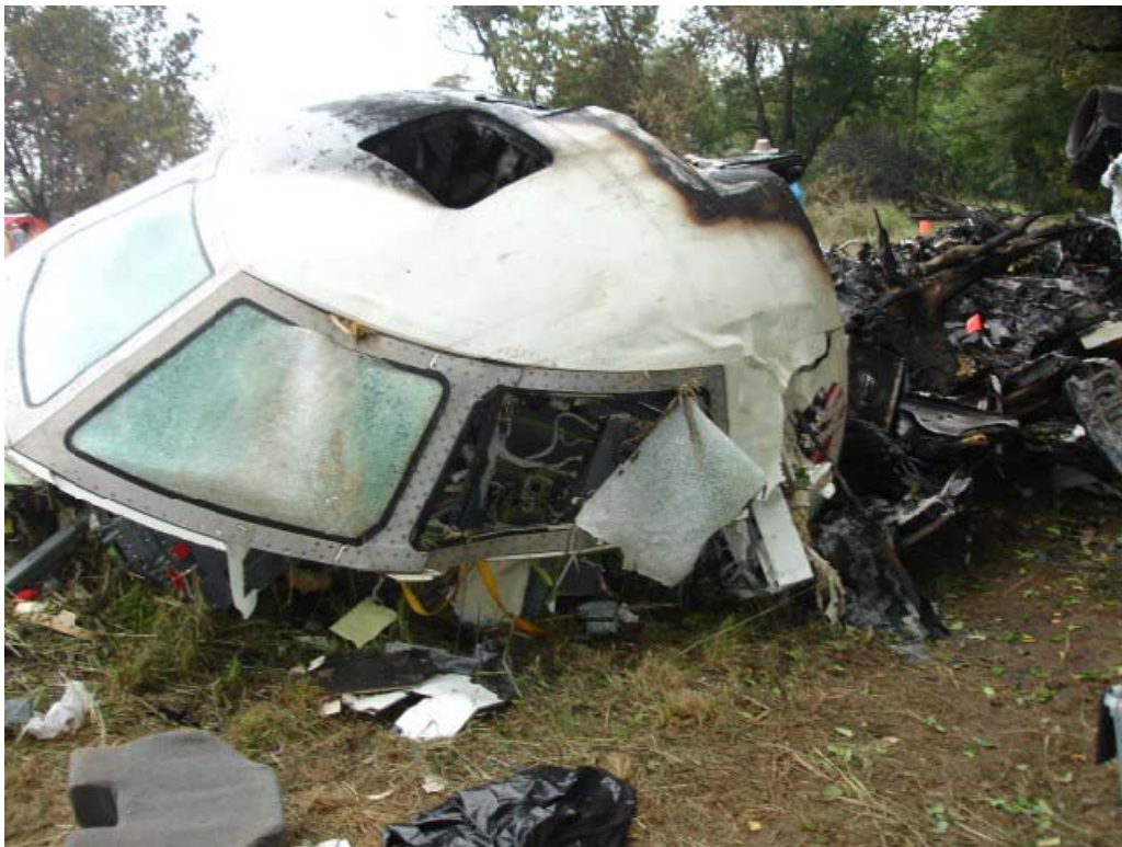
Photo 16. Cockpit damage and left side of the fuselage (note: main cabin door has been removed)
