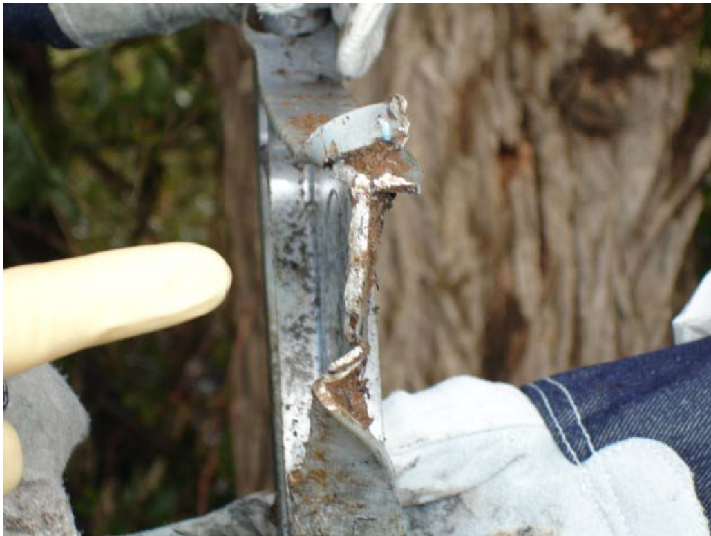
Photo 24. The fracture surface of the seat leg seen in photo 23
