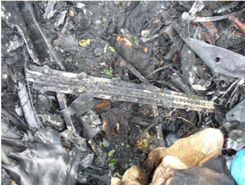
Photo 21. A section of fractured floor track
