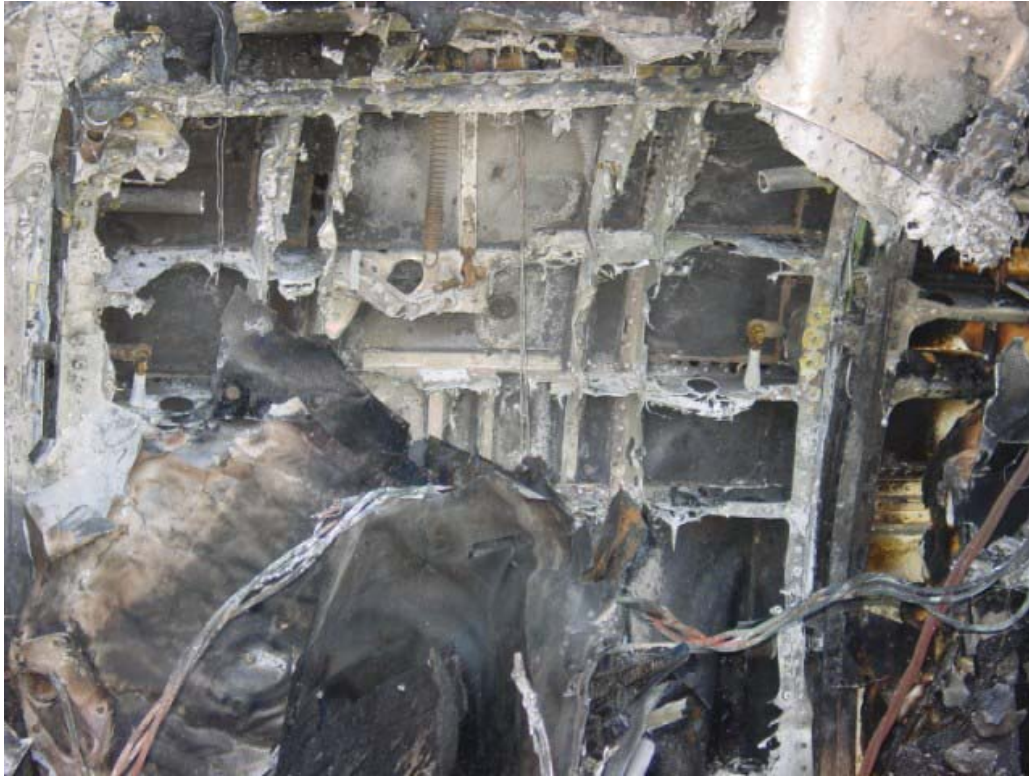
Photo 13. Interior of the main cabin door
