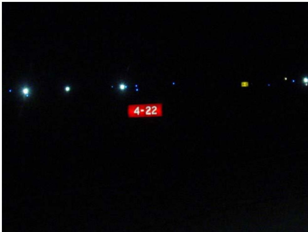
Photo 36. Runway 4/22 intersection sign as viewed from a 15-passenger van on the runway 26 centerline during the night taxi examination
