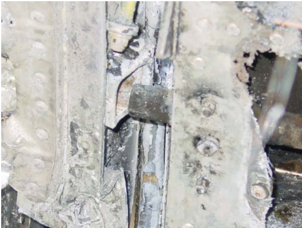
Photo 14. One of the main cabin door's extended aft lock pins
