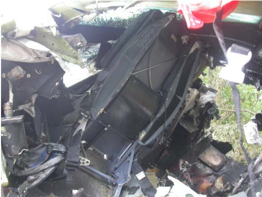
Photo 11. Portion of first officer's seat still attached to the cockpit floor structure
