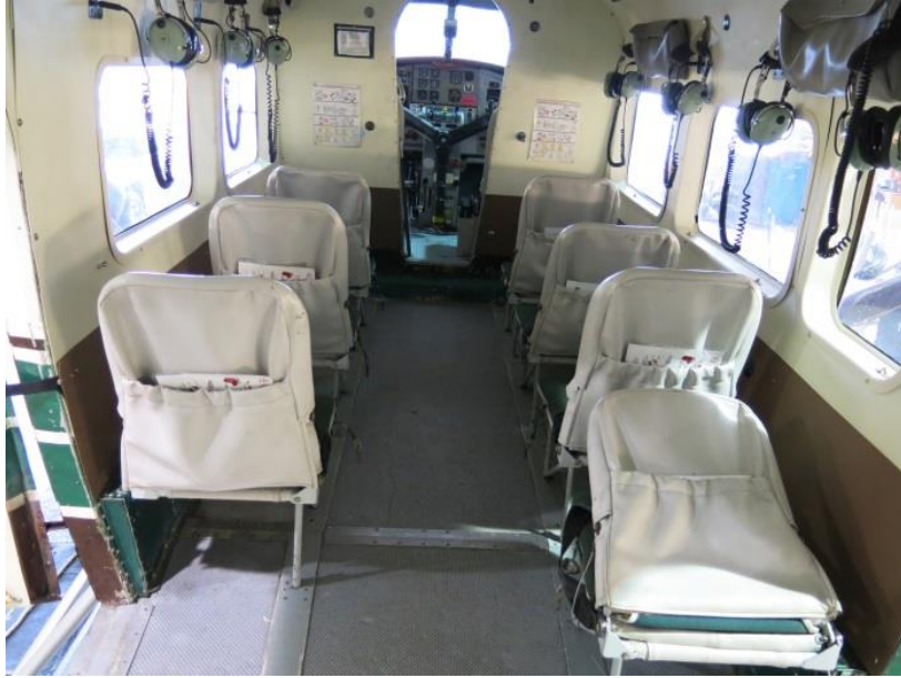
Photograph 3- Photograph of interior cabin standing aft looking forward toward the cockpit. R4 seat bent forward. Headsets stowed.
