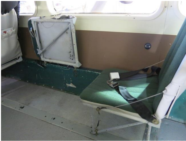
Photograph 10- Photograph of stowed cabin interior seat and a cabin interior seat in its downward and locked position.
