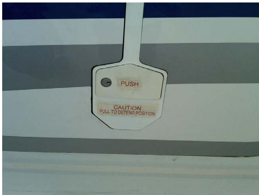
Photograph 8: Mechanical MED exterior release handle (from sistership).
