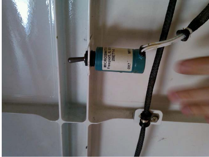
Photograph 5: Door opening toggle switch for test airplane mechanical MED (from sistership).
