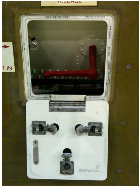
Photograph 18: Overwing exit exterior release handle (from sistership).
