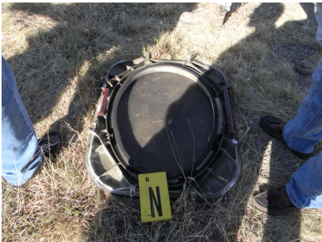
Photograph 14: Forward left overwing emergency exit position on-scene (Roswell, NM).
