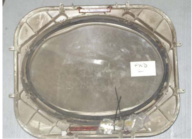
Photograph 22: Forward left overwing emergency exit door after accident (Lancaster, TX).
