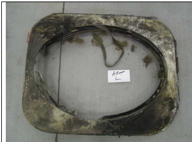
Photograph 19: Aft left overwing emergency exit door after accident (Lancaster, TX).
