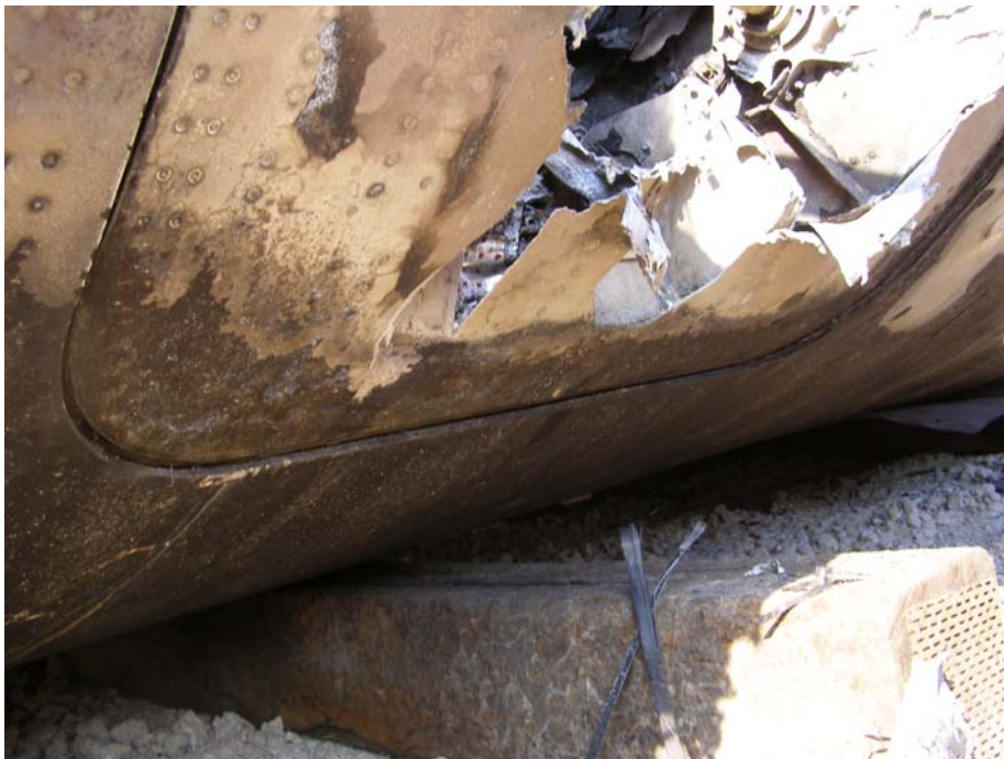
Photograph 12: Gap in lower portion of MED (Lancaster, TX).
