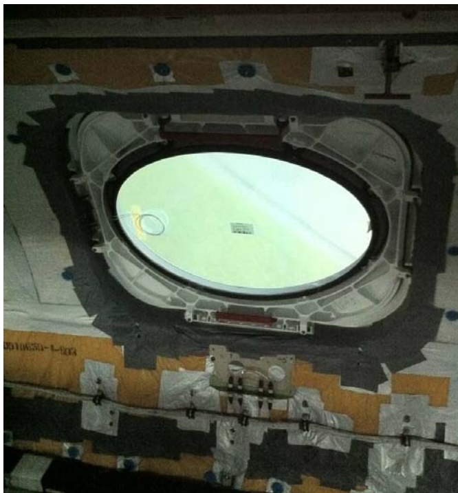
Photograph 15: Installed overwing emergency exit door from interior, T-handle in upper right (from sistership).
