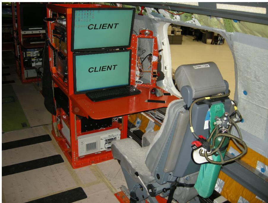
Photograph 2: Flight test engineer workstation with portable oxygen bottle and quick-don mask on seatback (from sistership).
