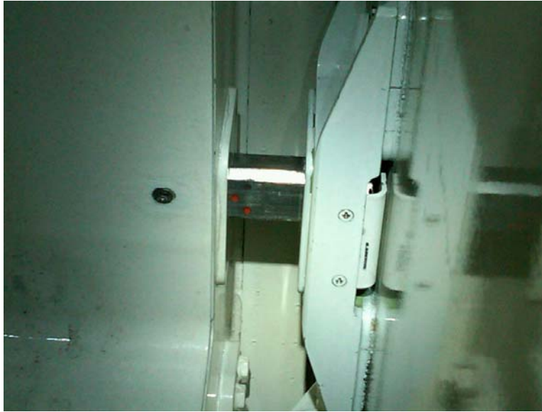
Photograph 7: MED locked indicator on bayonet (from sistership).
