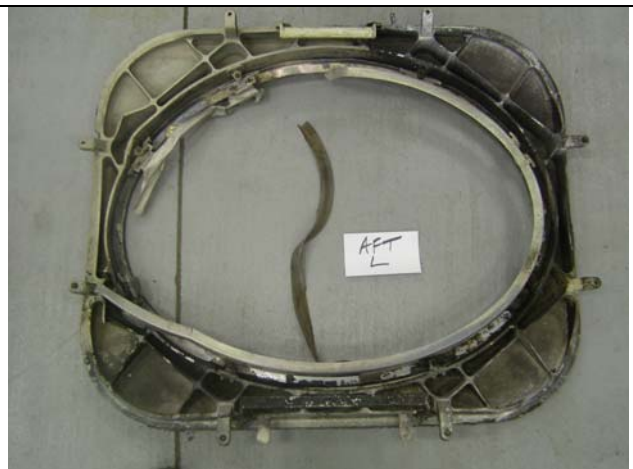
Photograph 20: Aft left overwing emergency exit door after accident (Lancaster, TX).
