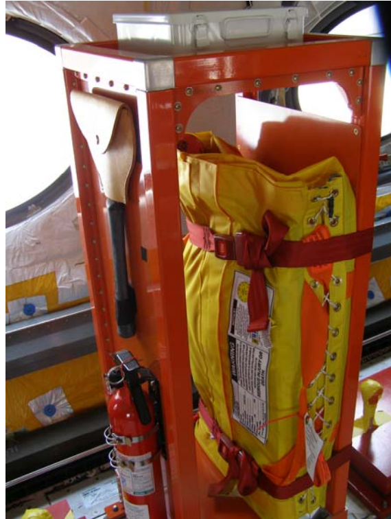
Photograph 1: Emergency equipment station (from sistership).
