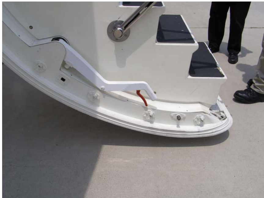
Photograph 6: Interior door release handle, unlock: red and unlatch: white (from sistership).
