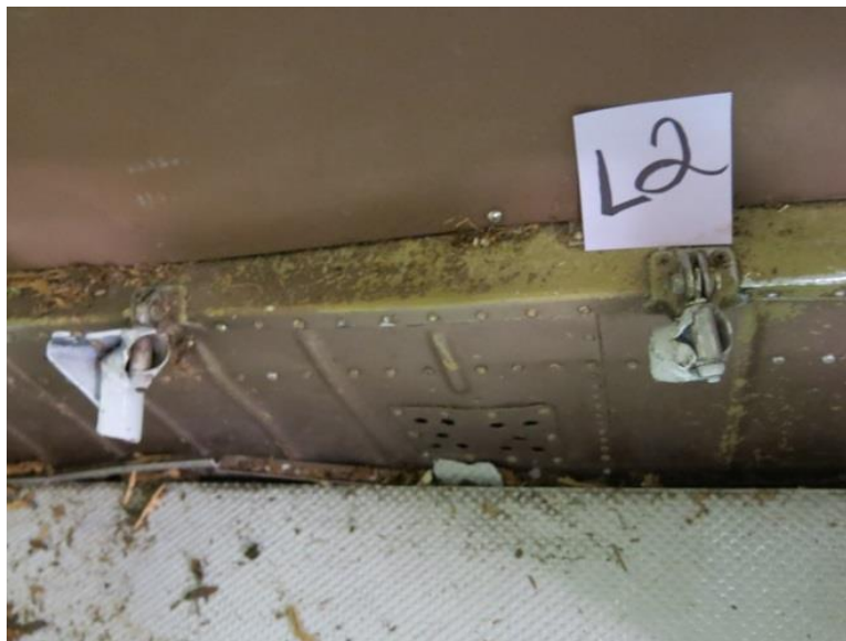
Photograph 12- Sheared L2 attachment points on the side of the fuselage.
