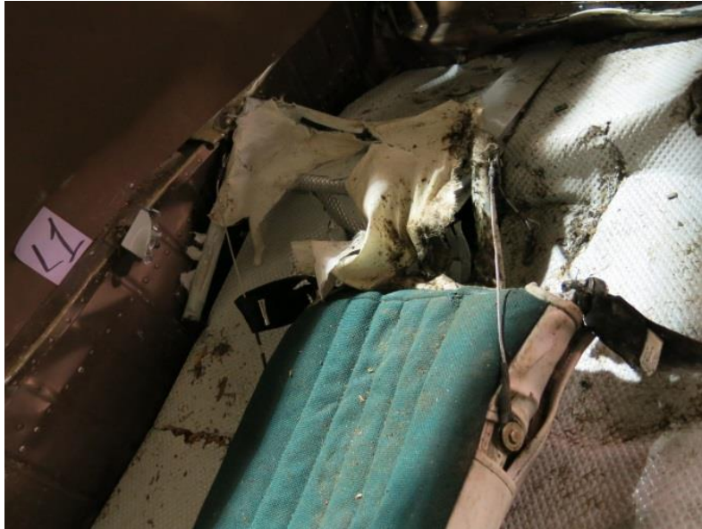
Photograph 10- Photograph of L1 seat bottom and deformation of the floor.
