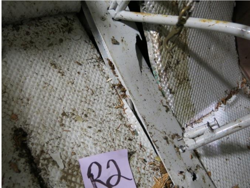
Photograph 25- Photograph of R2 seat legs and floor deformation.
