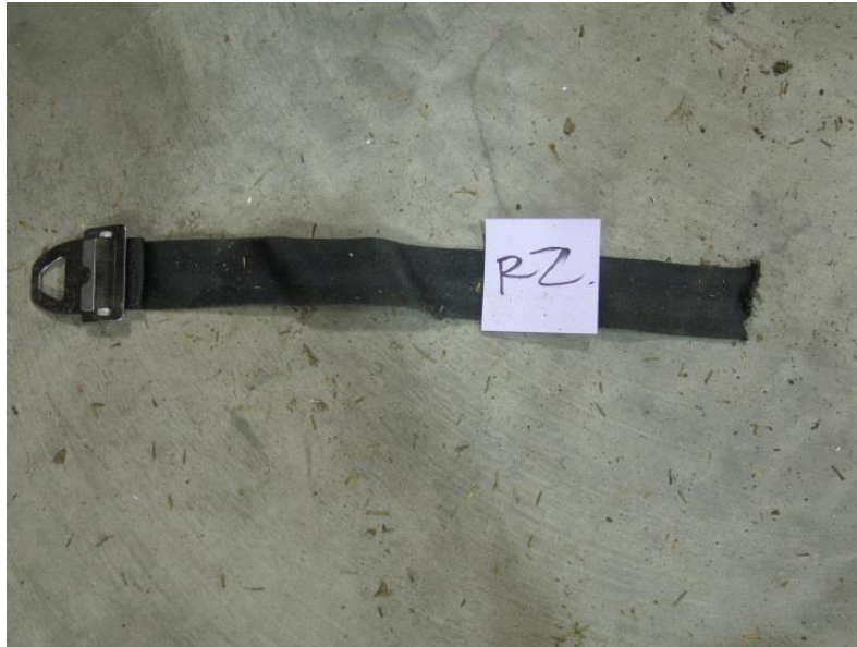
Photograph 23- R2 seat latchplate restraint. The restraint had been cut.
