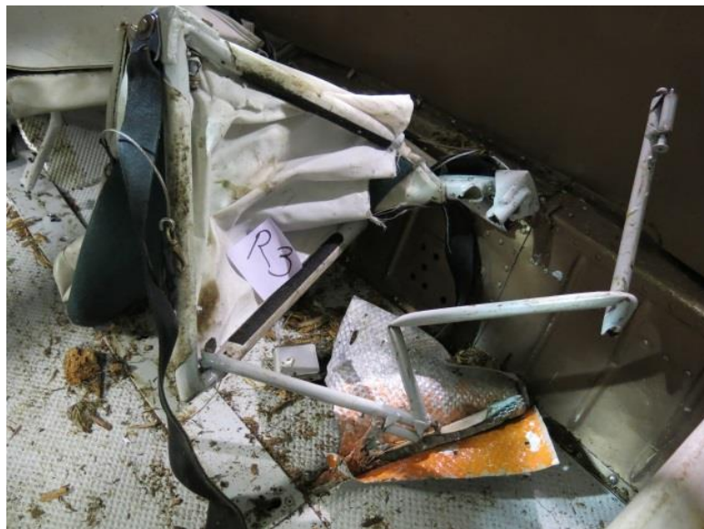
Photograph 30 - Photograph of deformed R3 seat.
