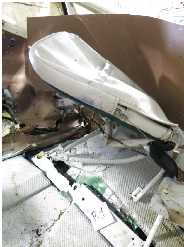
Photograph 22- Photograph showing R1 floor deformation, seatback, and seat legs.
