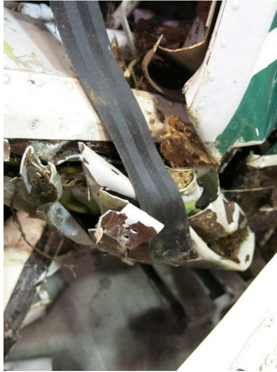
Photograph 5- Photograph of the cut seatbelt webbing at the pilot's seat.
