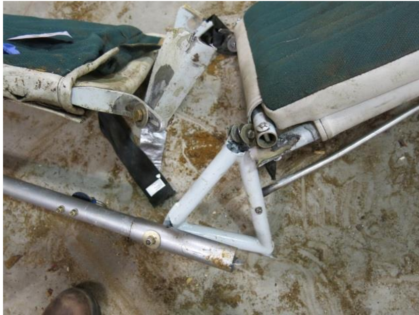
Photograph 16- Photograph showing L5 seat deformation.
