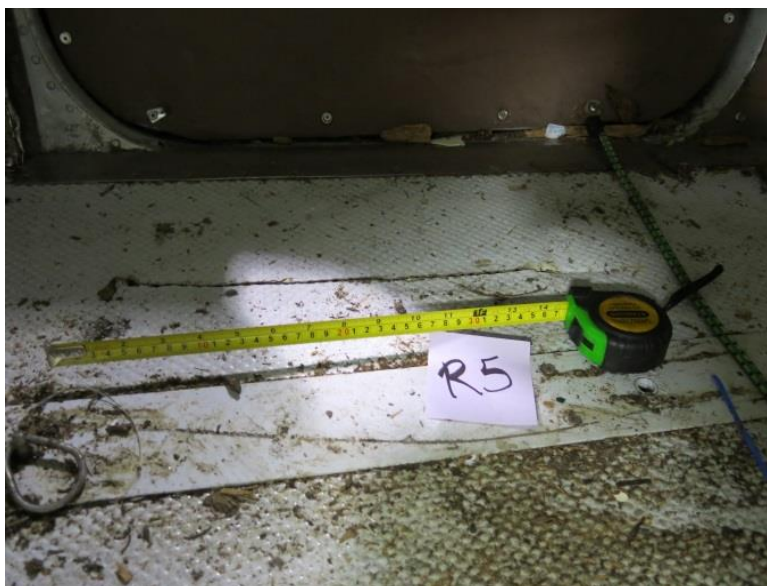
Photograph 39- Photograph of 13inch gash in the floor in front of R5 seat.
