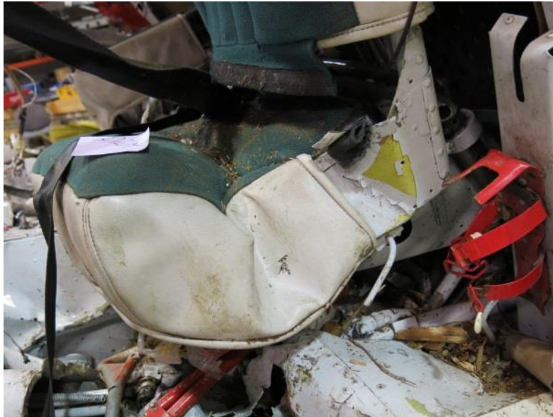
Photograph 3- Pilot seat showing deformation.
