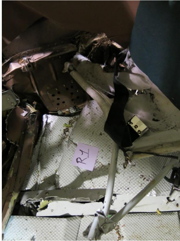
Photograph 20- Photograph of R1 floor deformation and seat legs.
