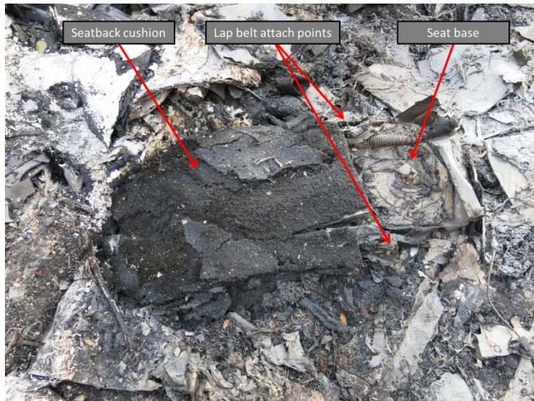
Photograph 5 – Passenger cabin seat consumed by fire.
