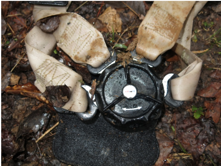
Photograph 2 – Pilot seat 4-point restraint.
