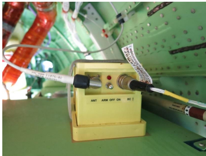
Photograph 2- Secured ELT inside the cargo compartment.
