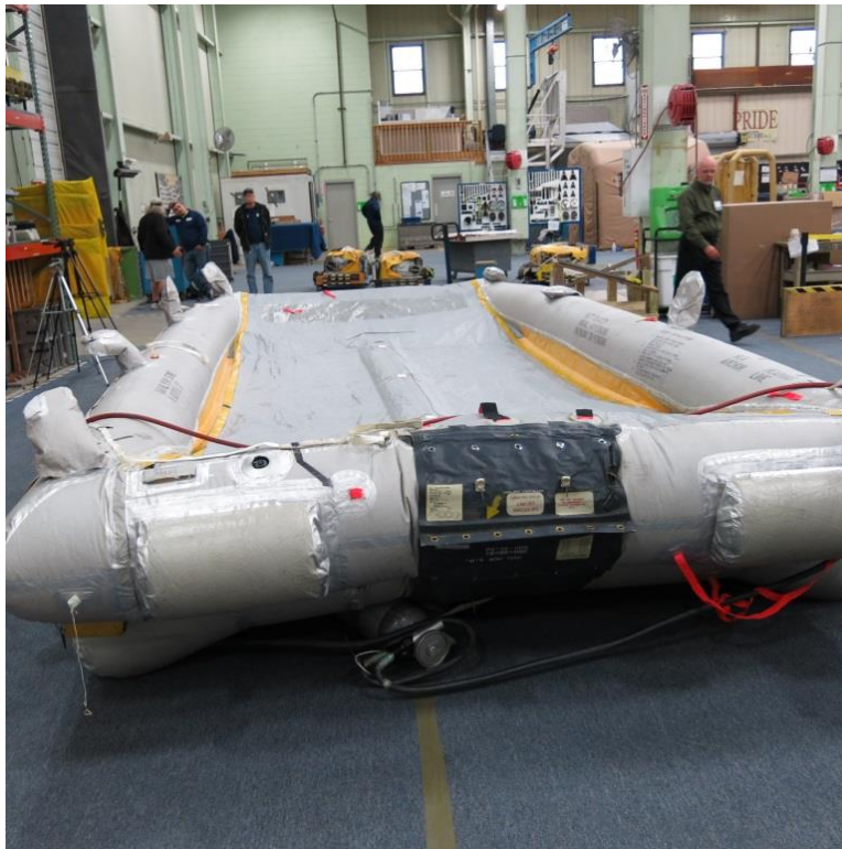
Photograph 9 -Slide/raft after flat fire test.
