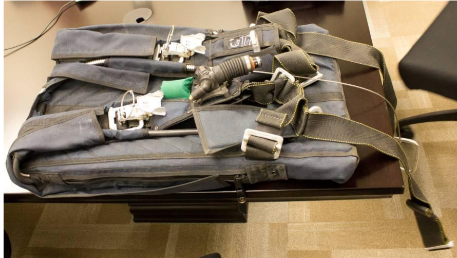
Pete Siebold's Parachute (Container with Oxygen Bottle Only)
