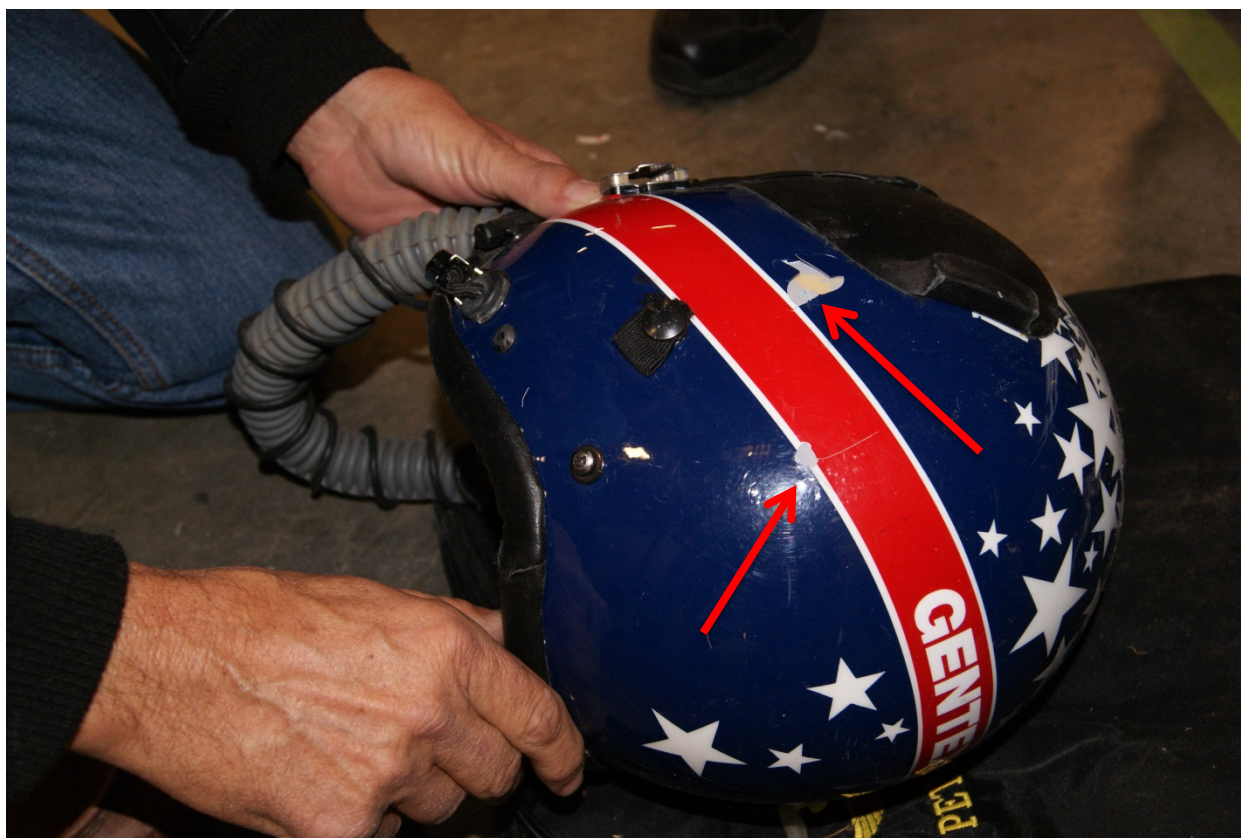
Photo 25. Pilot's helmet. (Note: two small areas of damage).
