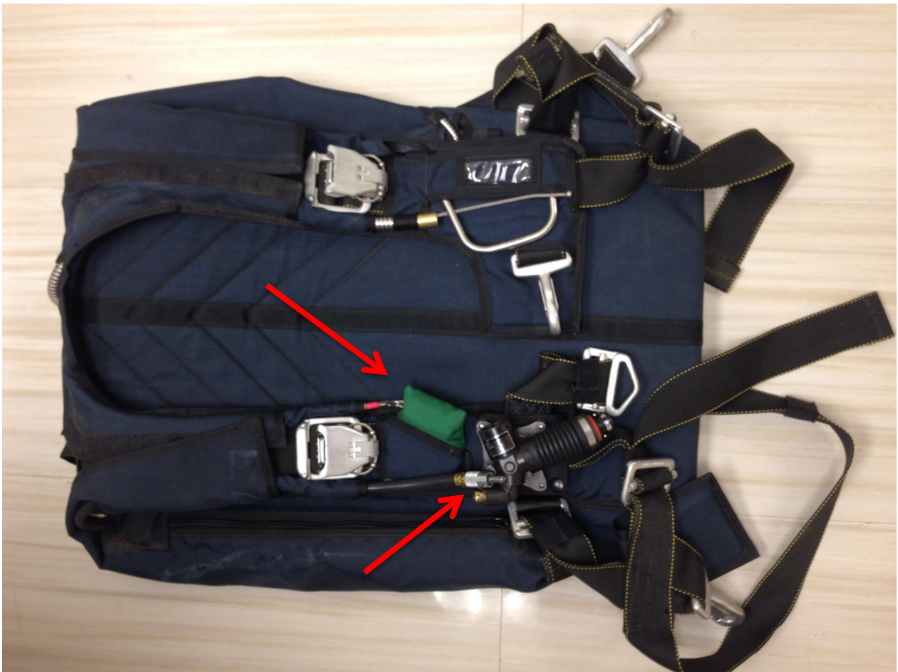
Photo 19. Pilot's parachute harness and container. (Note stowed green pad and disconnected oxygen hose.)
