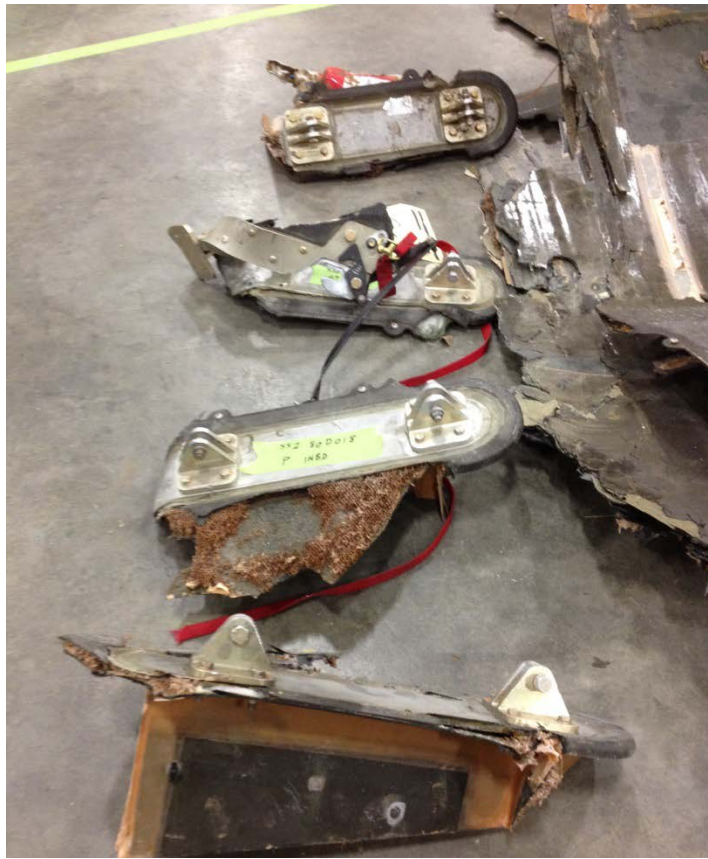
Photo 32. Floor fittings and floor plates from SS2.
