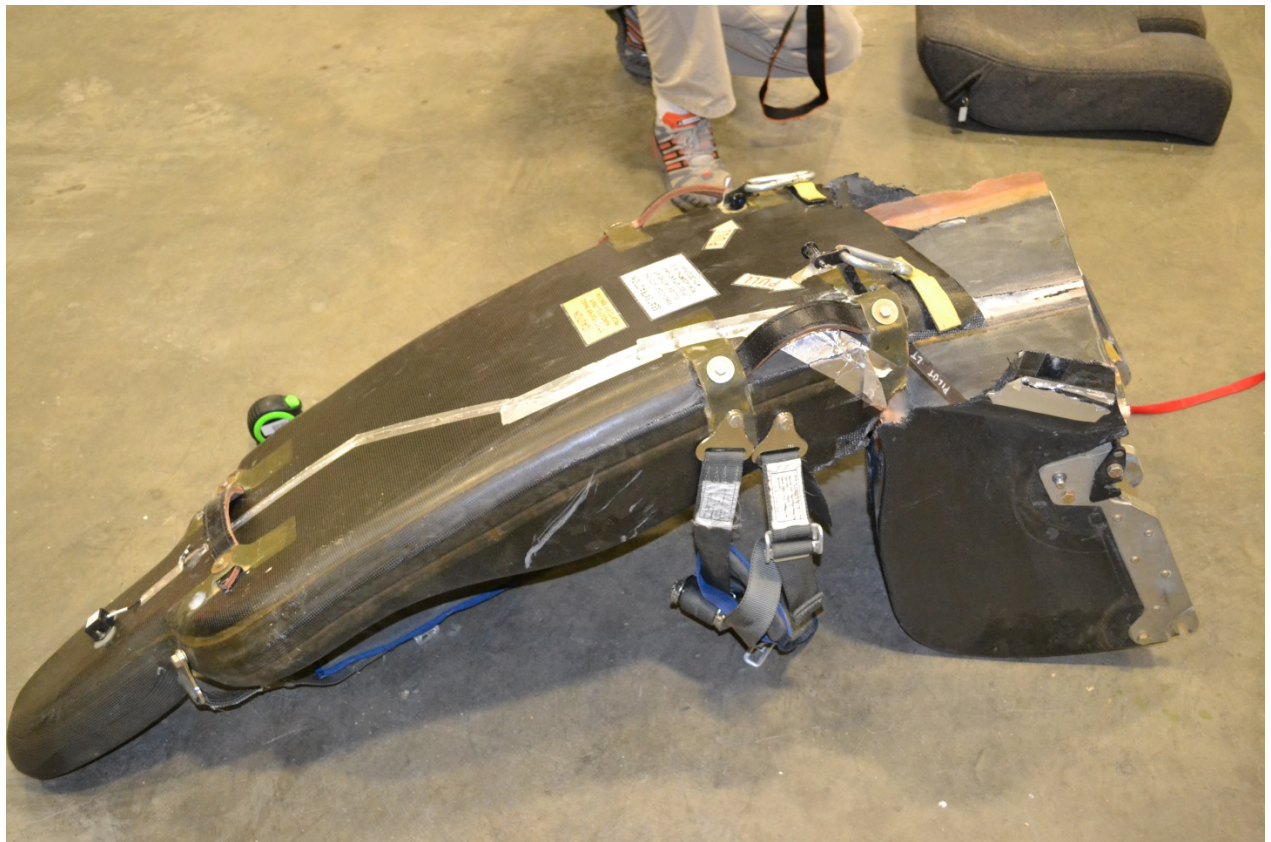
Photo 15. Pilot's seat as found by NTSB survival factors group.
