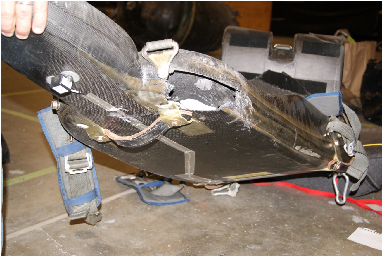
Photo 16. Damage to right shoulder area of pilot's seat.
