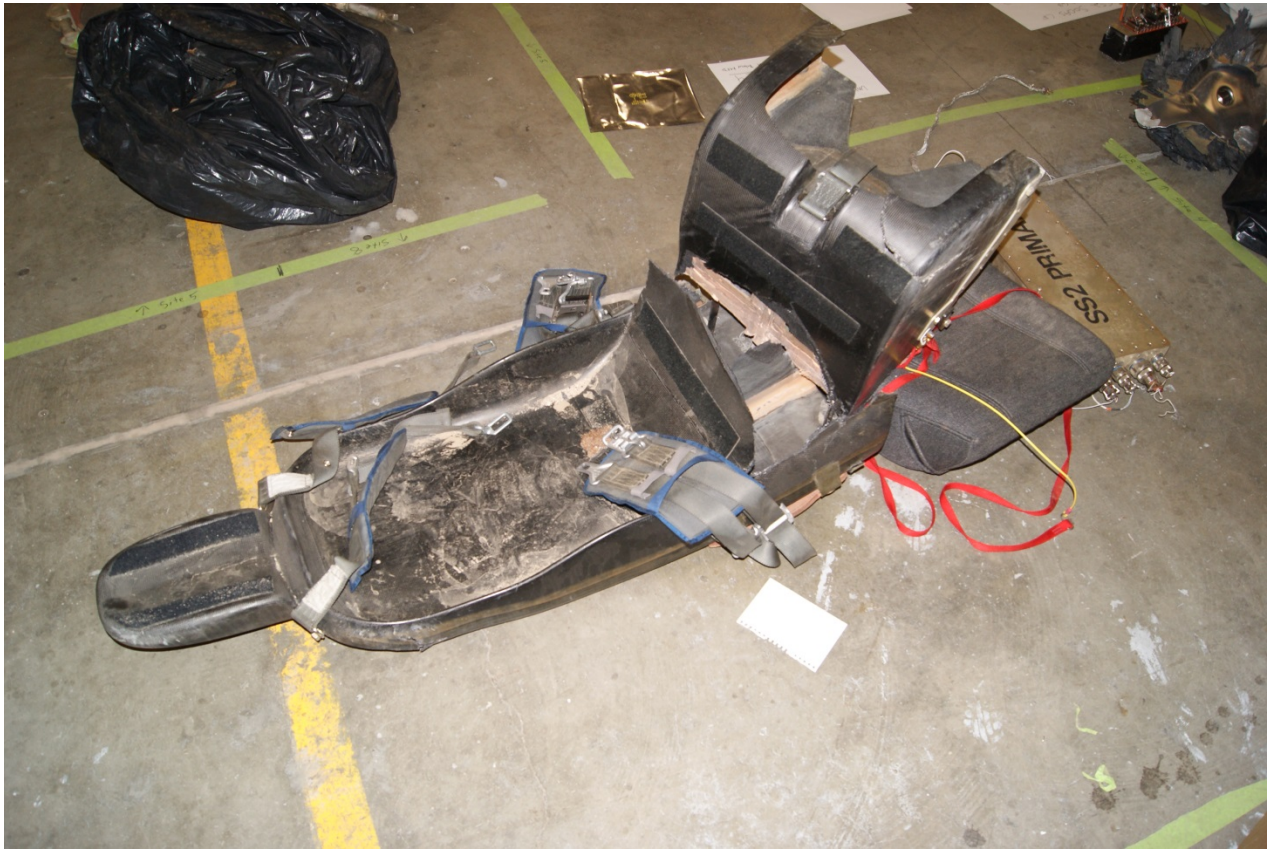
Photo 14. Pilot's seat as found by NTSB survival factors group.
