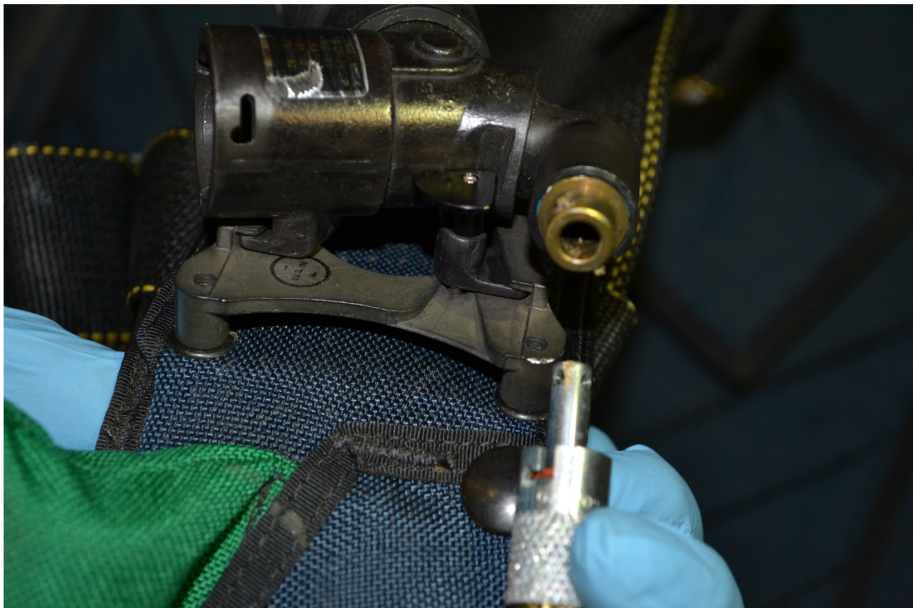
Photo 23. Close-up of disconnected oxygen hose.
