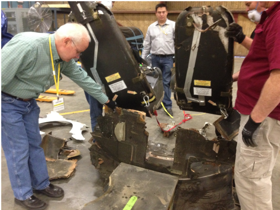
Photo 31. Reconstruction of raised pedestal, crew seats, and flooring of SS2.
