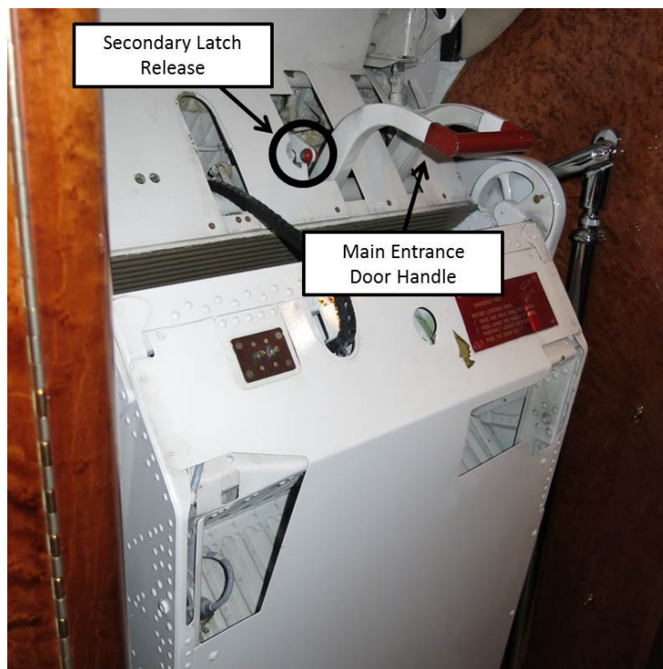
Photograph 16. G-IV main entrance door interior handle and secondary latch release.
