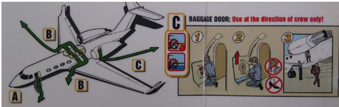
Figure 2. Excerpt from passenger safety information card showing the baggage door supplementary emergency exit.
