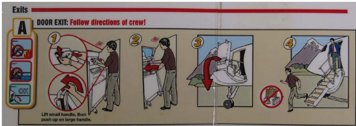
Figure 6. Excerpt from the passenger safety information card showing main entrance door operation.
