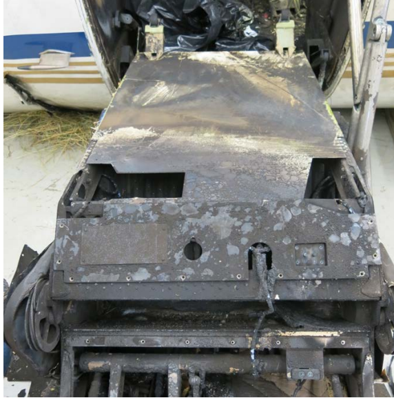
Photograph 20. Main entrance door stair folded at over center latch.
