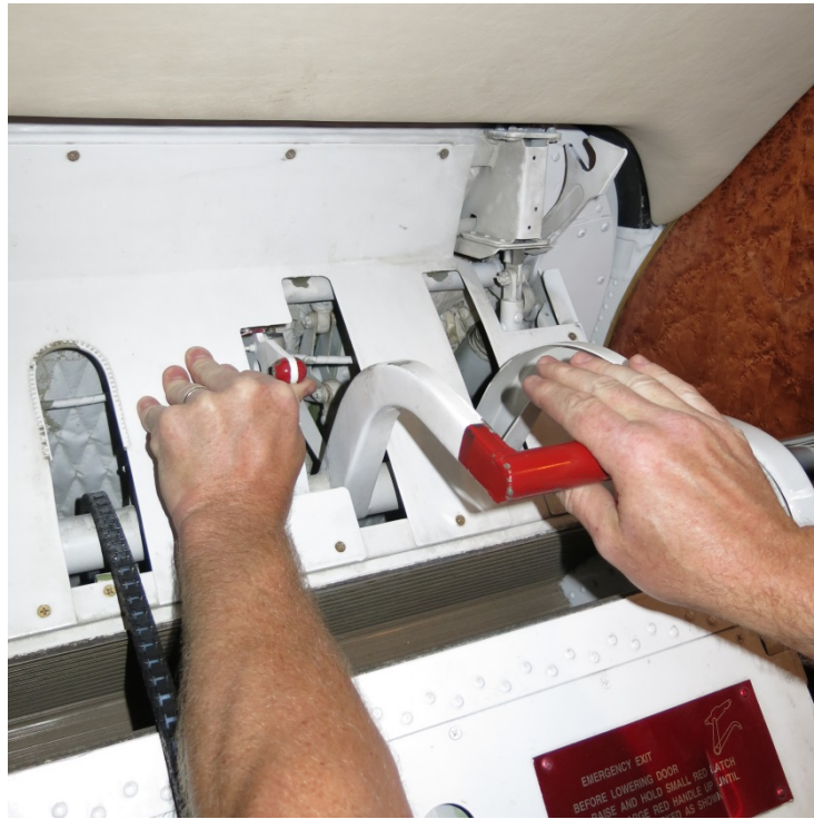
Photograph 17. G-IV main entrance door opening procedure.
